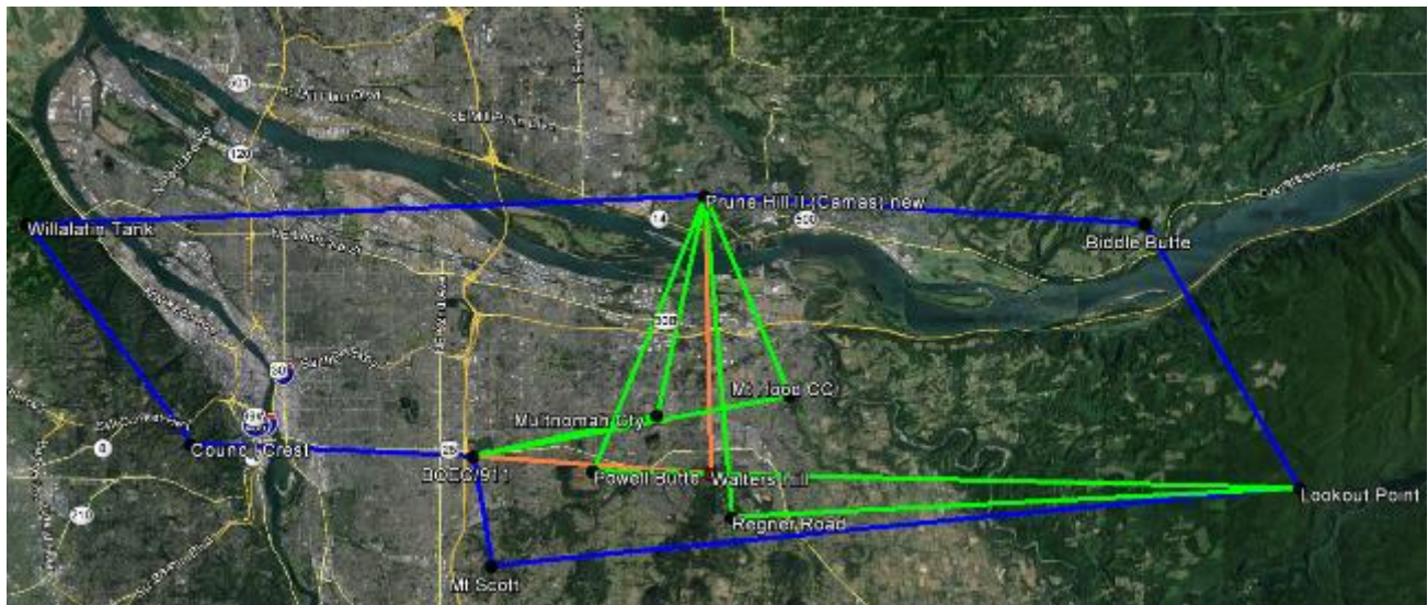
Figure 1 – Potentially Suitable Alternate Site Microwave Radio Paths and Motorola-Proposed Microwave Radio Ring
