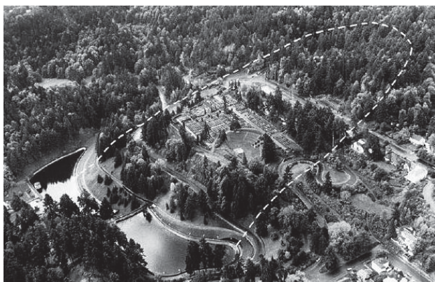
Figure 6. Outline of ancient landslide (Turner Schuster)
