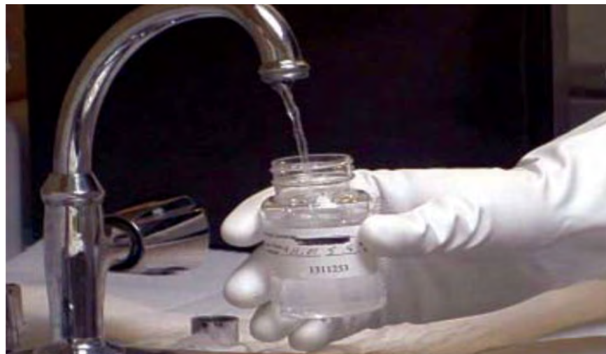
EPA water sampling procedure using gloves as contaminant barrier and controlled flow
