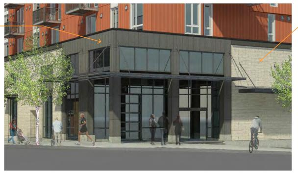
Arriscraft Masonry changed to Brick to simplify material palette
