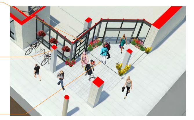
Area for retail spill out increased, Depth of recess increased 1.5' to 14.5'
