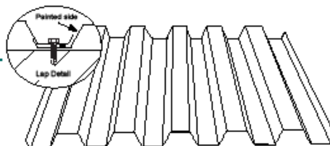
Reversed HR-36 Wall (typical wall applications)
