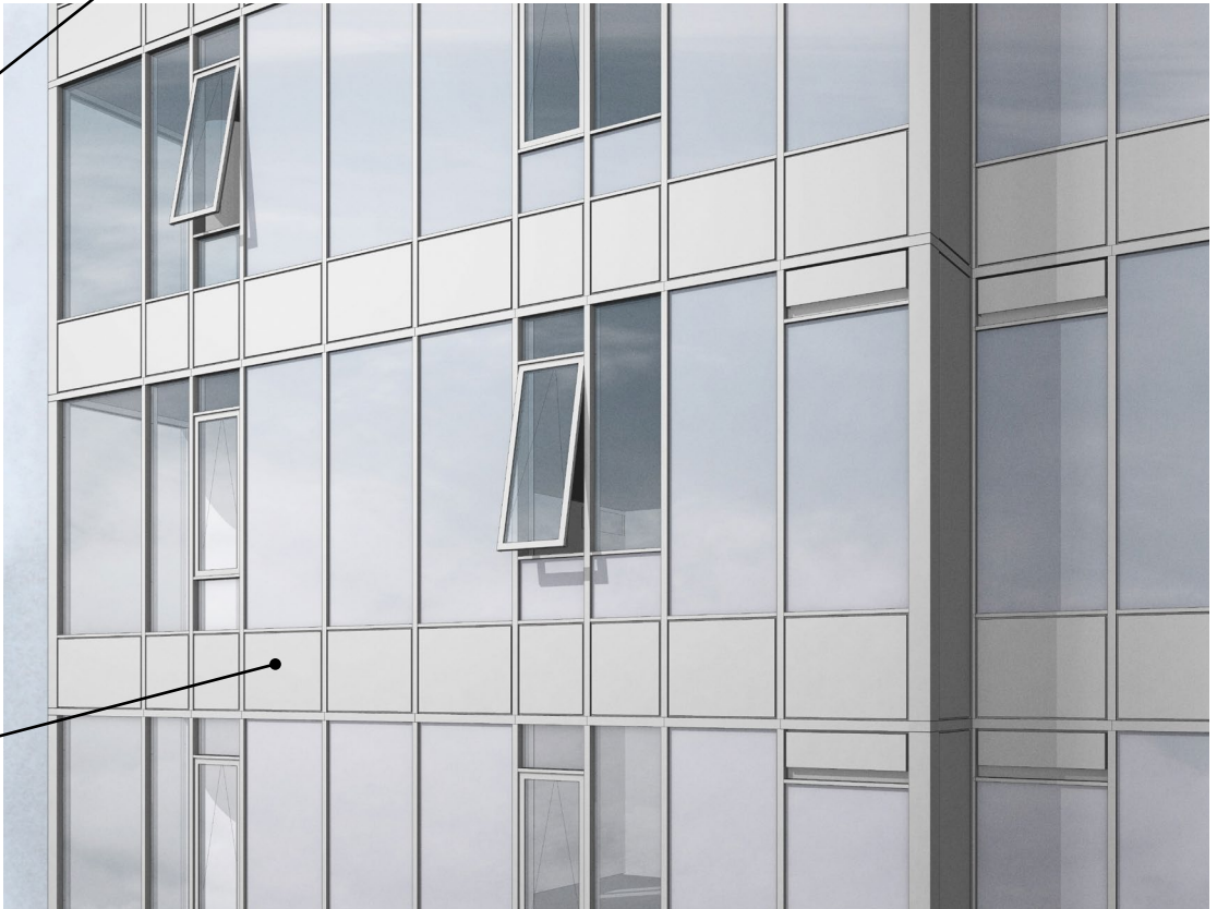
Painted Metal Panel at tower body "Light Grey" to match PPG "Satin Nickel" or simi- lar. To be used at slab edge, louver, and mullion.
