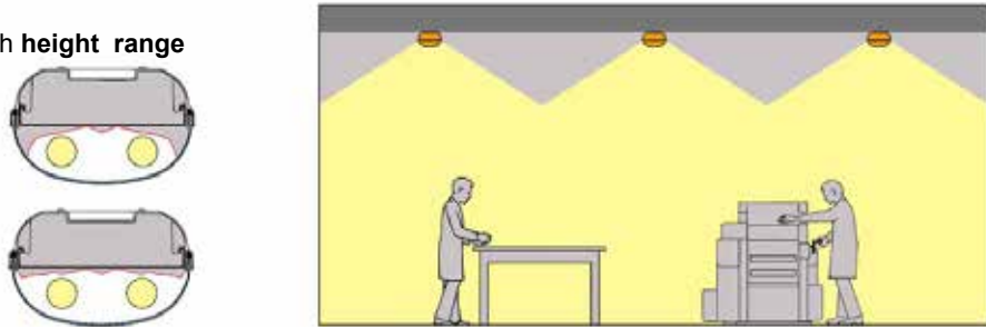
Parabolic flow reflector wide direct distribution, for luminaires 6 inches wide.
