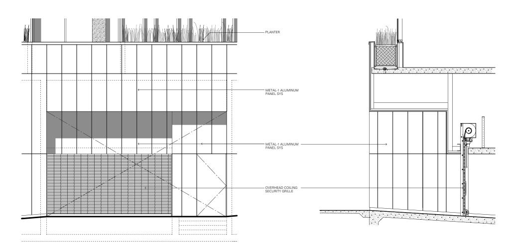
Enlarged Elevation: East Garage Gate
