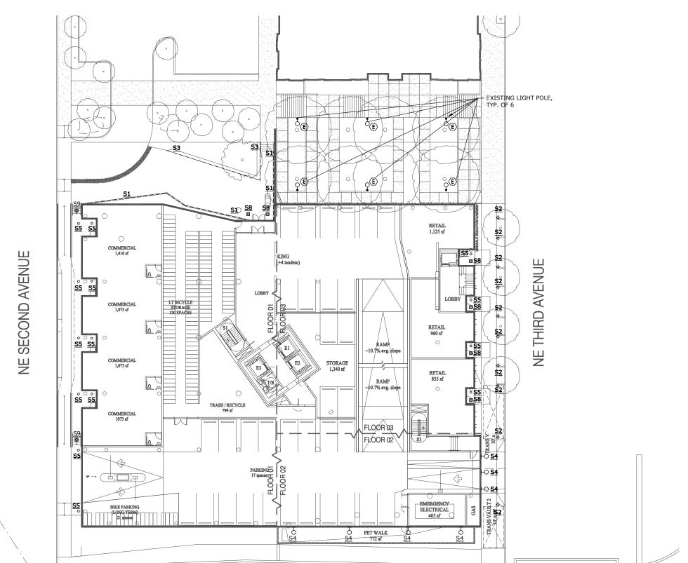
LUMINAIRES: S1 - LED LINEAR STATIC WHITE OR COLOR S2 - LED ILLUMINATING BOLLARD S3 - LED FLEXIBLE LINEAR
