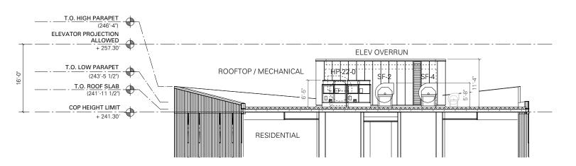
Enlarged Section (Tower Roof) 1/16"=1'-0"
