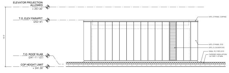
Enlarged Elevation (Elevator Overrun - North) 1/8"=1"-0"
