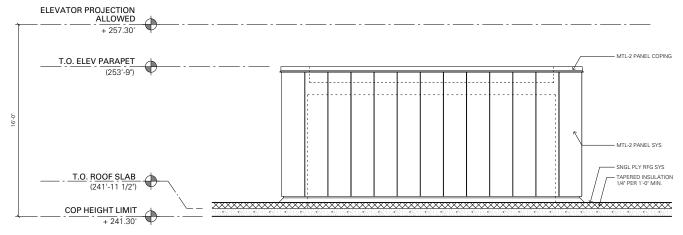
Enlarged Elevation (Elevator Overrun - West) 1/8"=1'-0"
