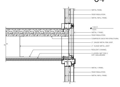
ALT TOWER STRUCTURE - METAL PANEL TO METAL PANEL 03
