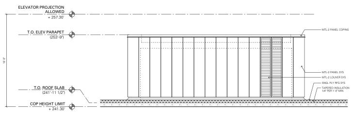
Enlarged Elevation (Elevator Overrun - South)
