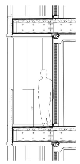
ENLARGED SECTION AT TOWER BALCONIES - B3 (B4 SIM)
