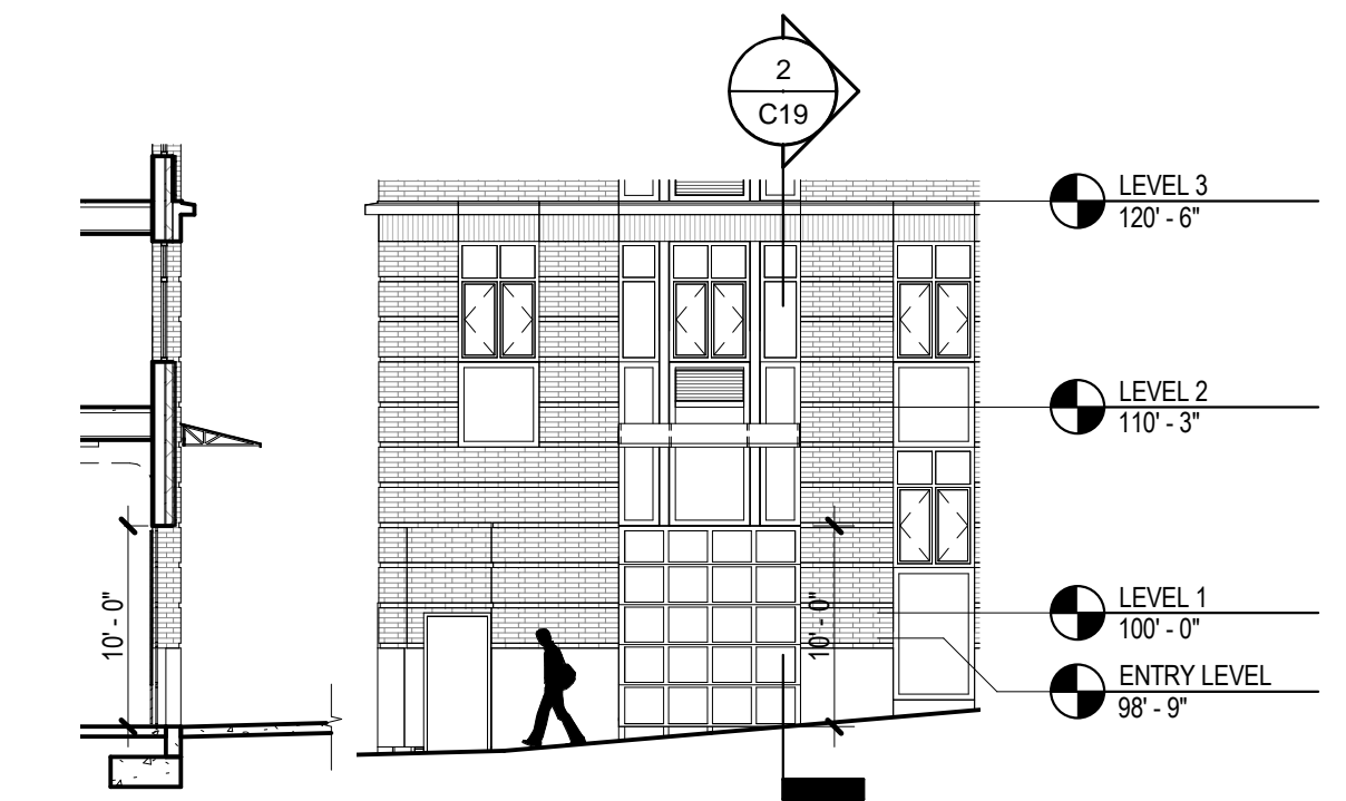
WALL SECTION 2 ENLARGED LOADING ELEVATION 1
