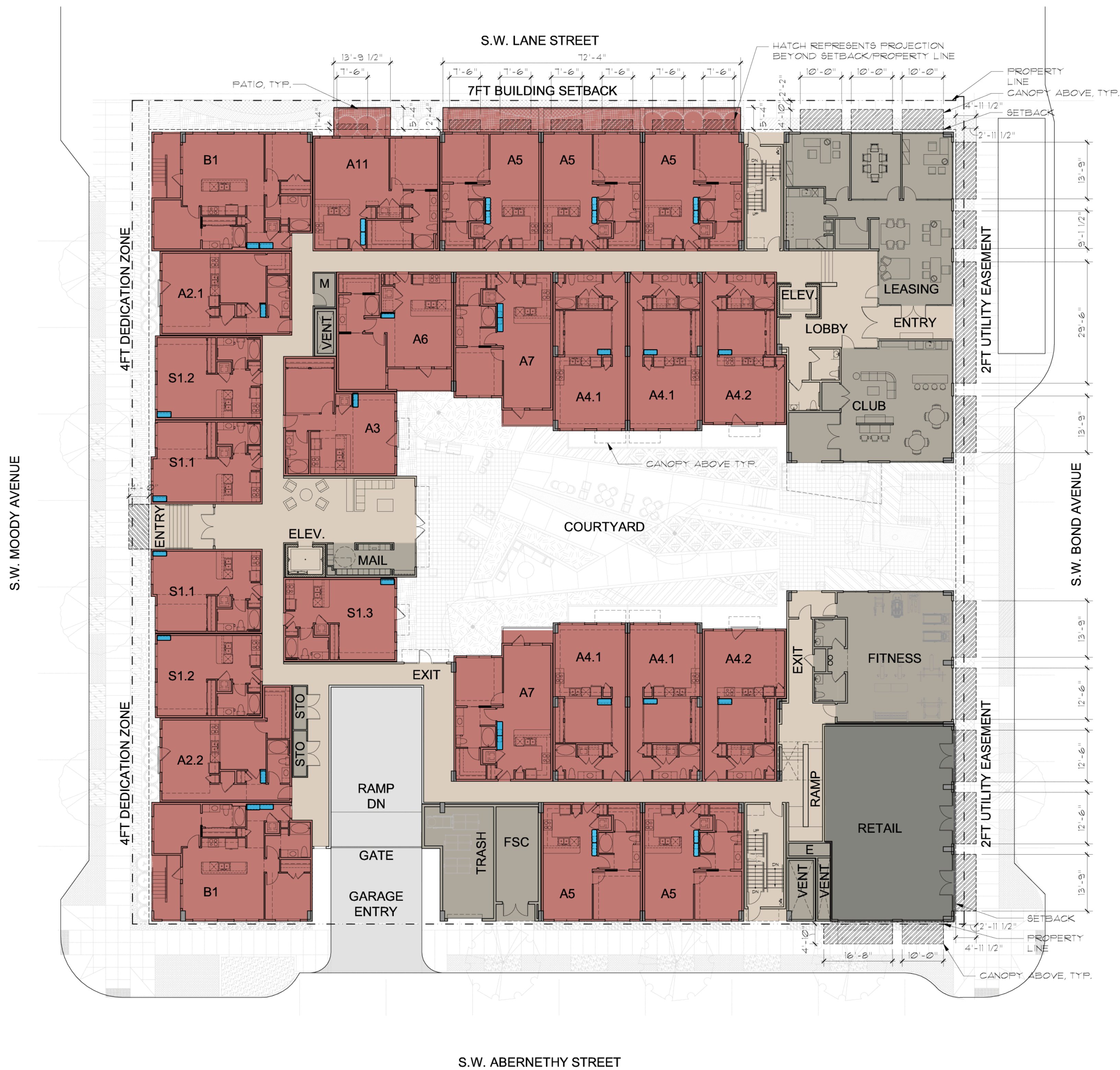
FLOOR PLAN UNIT LEVEL 1 SCALE: 1/16" = 1'-0"
