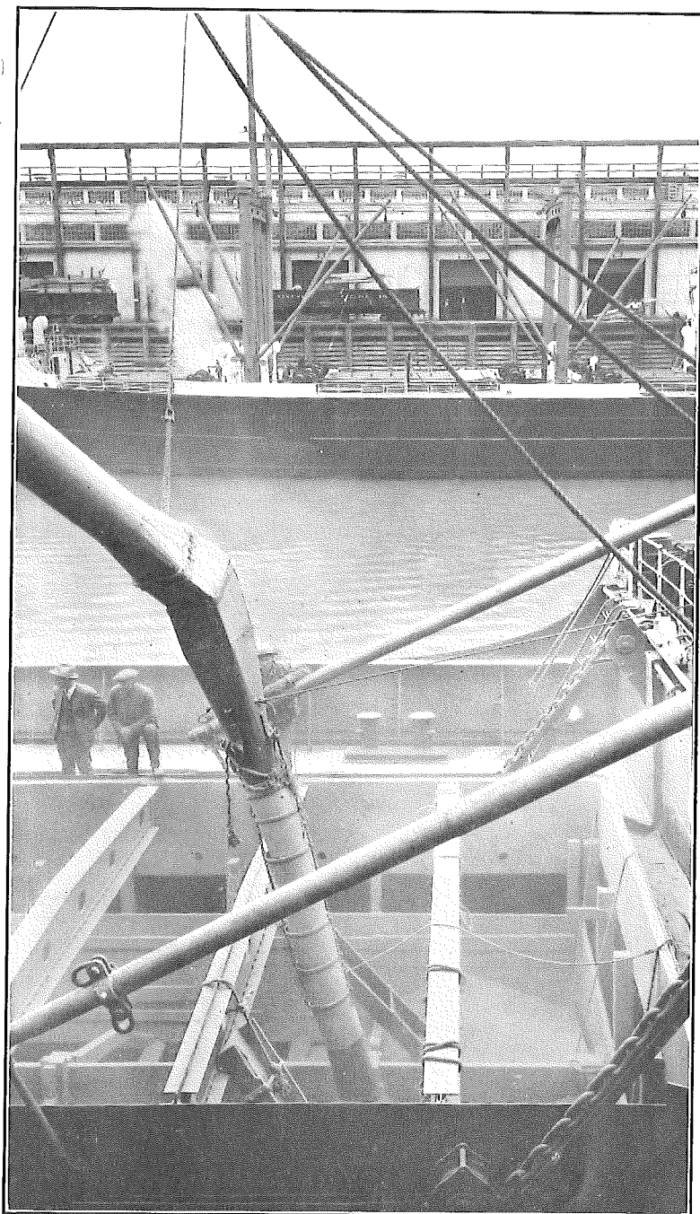
SPOUTING BULK GRAIN FROM GRAIN ELEVATOR INTO VESSEL'S HOLD AT PIER NO. 1, MUNICIPAL TERMINAL NO. 4
