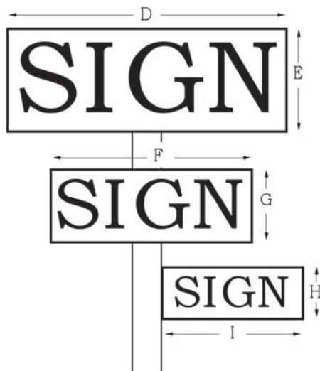
Figure 4 Sign Face Measurements
