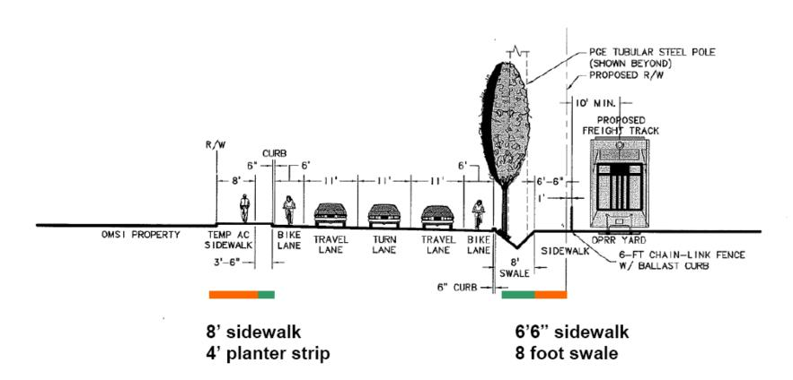
Note: Revised section is conceptual only. Design requirements for swale sizing and PGE pole placement still being developed.
