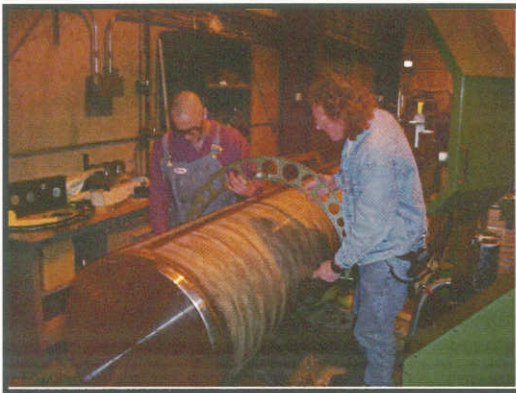
Large Micrometer Inspection of Diameter to +/- .001"
