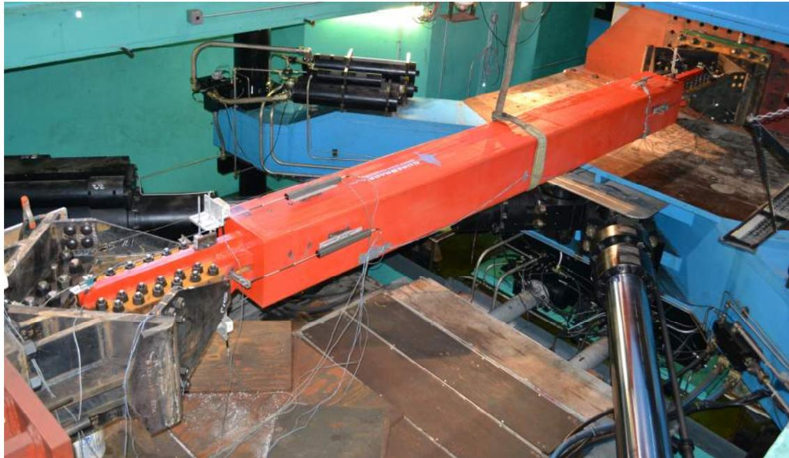
Figure 3.47 Specimen 5P: Test Setup
