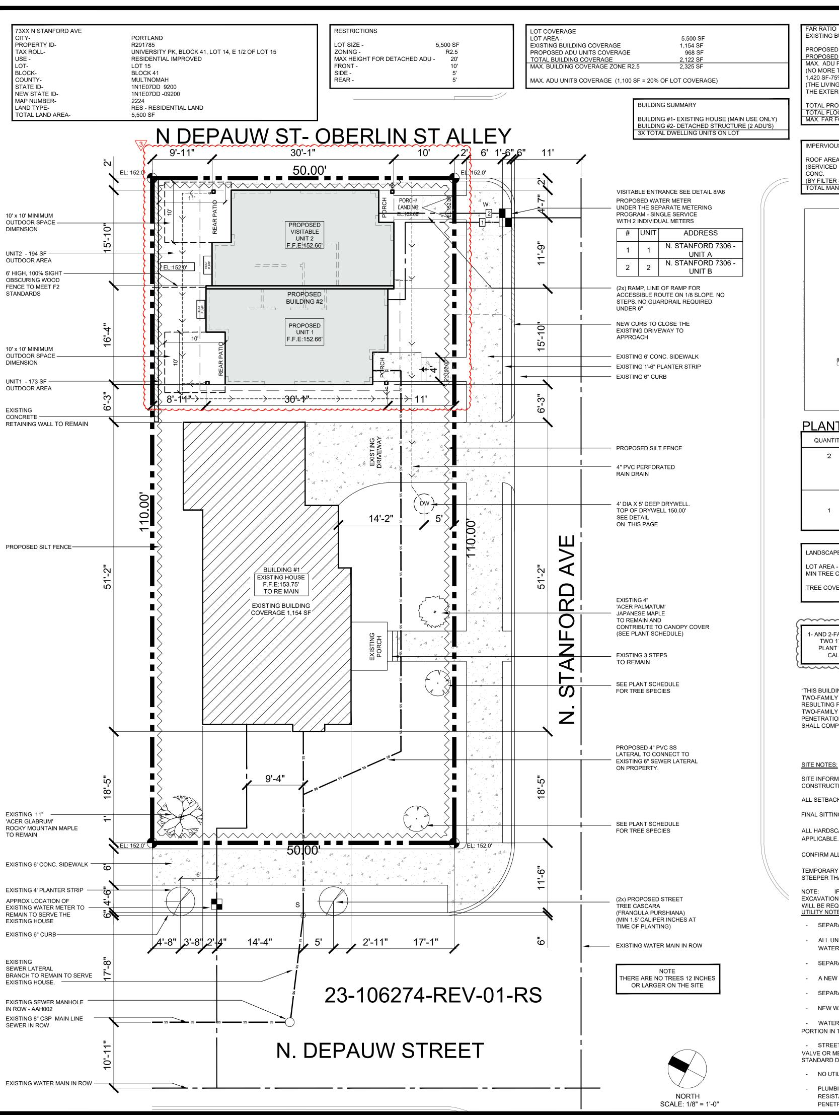
EXISTING BUILDING LIVING AREA 1,420 SF 796 SF PROPOSED ADU UNIT 1 LIVING AREA PROPOSED ADU UNIT 2 LIVING AREA 796 SF (NO MORE THAN 75% OF THE LIVING AREA OF THE PRIMARY STRUCTURE 1,420 SF-75%= 1,065SF (OR LARGER OF TWO UNITS IN A DUPLEX) OR 800 SQUARE FT THE LIVING AREA IS CALCULATED BY EXCLUDING THE THICKNESS OF THE EXTERIOR WALLS) OTAL FLOOR AREA MAX. FAR FOR R2.5 ZONE (3 UNIT FAR 0.9:1)
