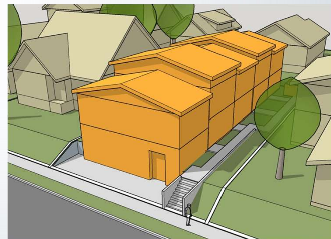
Excavation to bring unit to sidewalk level
