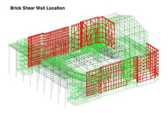
To help understand a rough order of magnitude of the necessary upgrades, Miller developed an engineering cost estimate. This estimate was based on repairs to strengthen the concrete and masonry walls adding reinforced pneumatically placed concrete to the inside face of the wall to resist the missing shear capacity, as well as provide additional out-of-plane capacity. Masonry partition walls were expected to either be braced or removed and replaced with metal stud walls.
