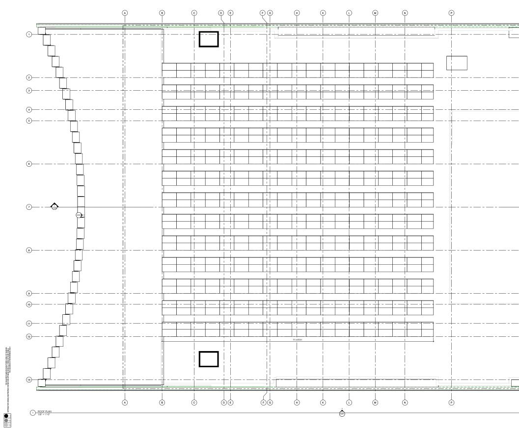
ROOF PLAN LEGEND THE FOLLOWING SYMBOLS ARE SHOWN ONLY WHERE LAYOUT IS CRITICAL FOR AESTHETICS. THE ACTUAL DESIGN MAY CALL FOR MORE THAN WHAT IS SHOWN. NOT ALL SYMBOLS MAY BE USED. O DOWNSPOUT ROOF DRAIN AND OVERFLOW DRAIN SLOPE ROOF SLOPE ( 1/4" / 12" MIN.)
