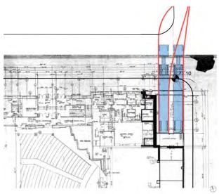
This plan illustrates the truck loading path impacts to the right-of-way
