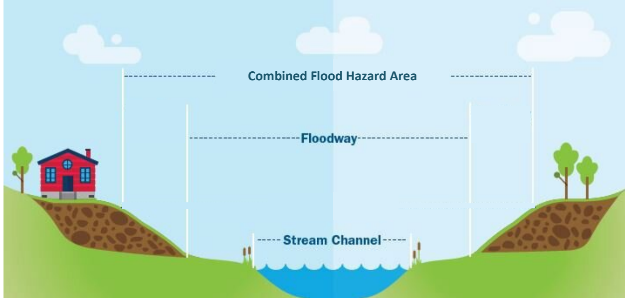
Figure showing generalized cross section of the waterbody (stream), floodway, and combined flood hazard area
