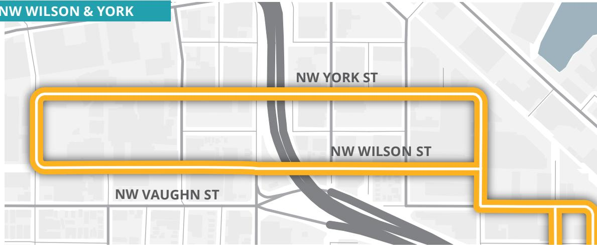
In Northwest, the proposed streetcar extension alternative would operate on NW York and NW Wilson Street. The streets in the area are not uniform, with many lacking typical sidewalks, formalized parking, and bike facilities. The alignment shown would rely on the City of Portland gaining easements and right-of-way from private property owners. For example, today NW York Avenue terminates at NW 24th. One block of NW Wilson street between 24th and 25th is also privately owned.
