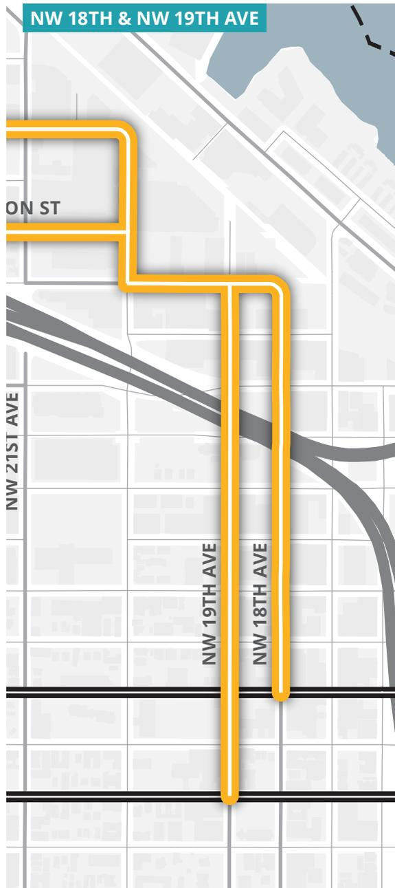
The streetcar extension alternative operates on NW 18th and 19th to tie into the existing streetcar line at NW Northrup and NW Lovejoy. NW 18th and 19th form a couplet, a bike buffered bike lane, and a vehicle lane shared with buses. Twelve foot sidewalks are separated by a landscape strip or street furniture. The full right of way is approximately 60 feet.
