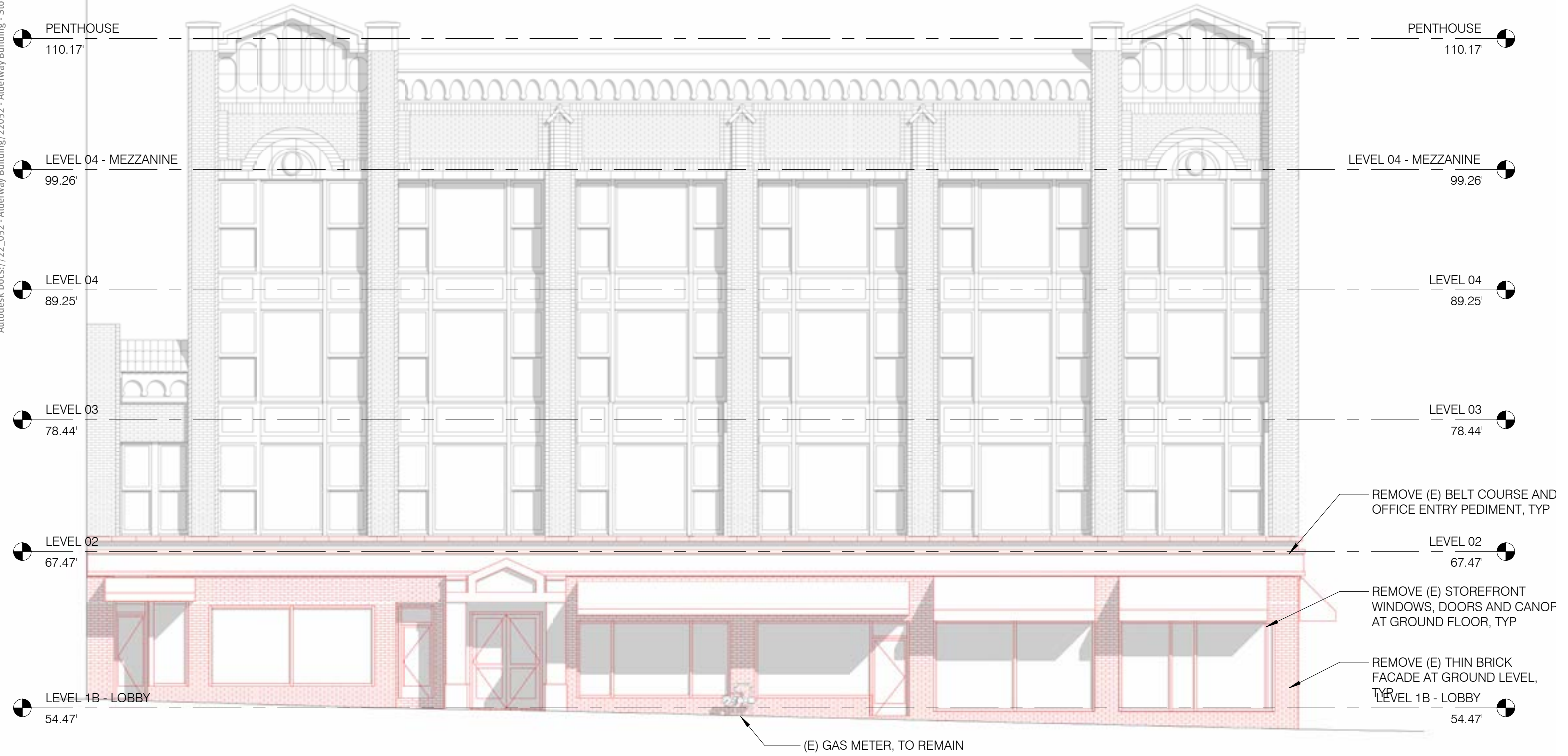
1 EXISTING ELEVATION - SOUTH - DEMOLITION 1/8" = 1'-0"
