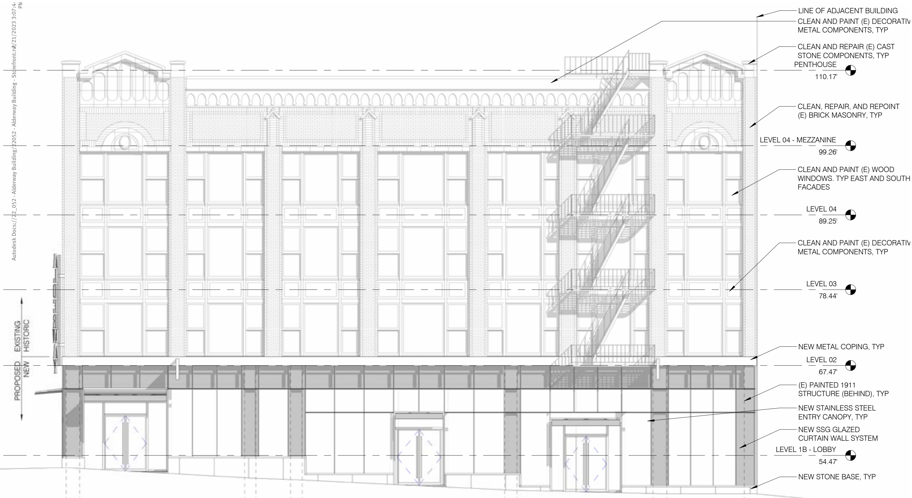
2 EAST ELEVATION 1/8" = 1'-0"
