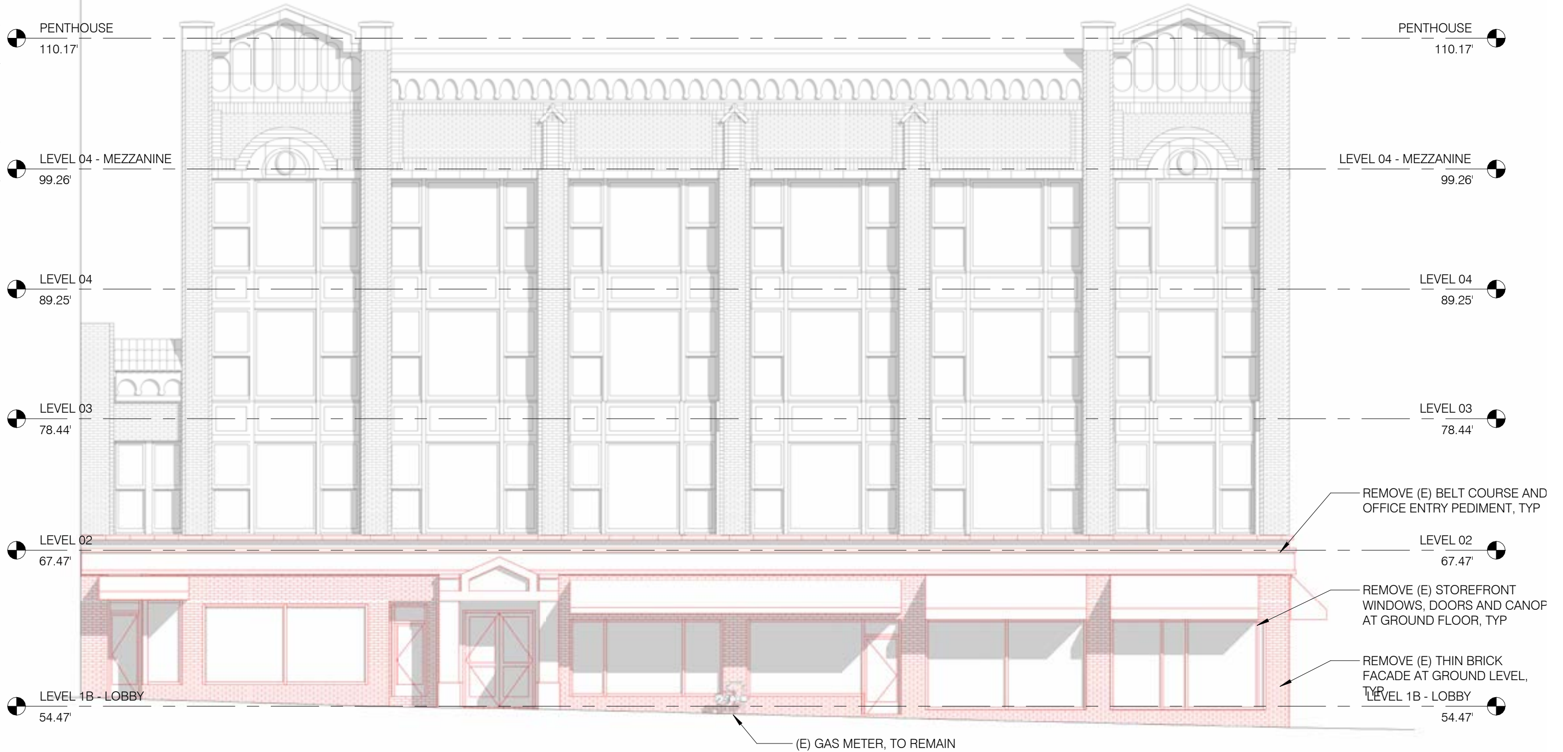
1 EXISTING ELEVATION - SOUTH - DEMOLITION 1/8" = 1'-0"
