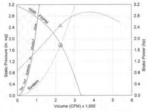
Operating Bhp point Operating point at Total SP Operating point at External SP Fan curve - - - System curve
