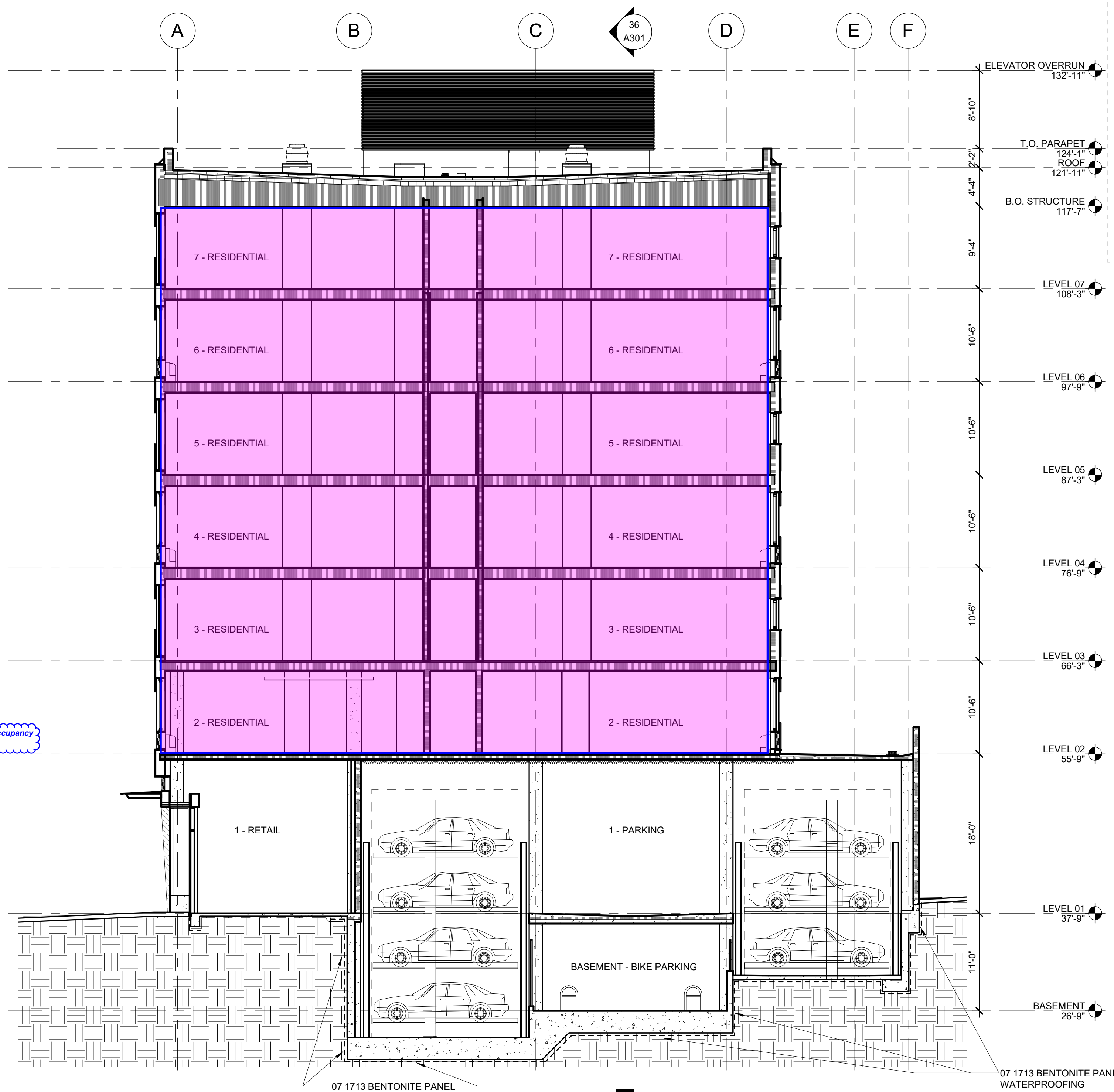
15 EAST-WEST BUILDING SECTION LOOKING NORTH AT STACKER PIT
