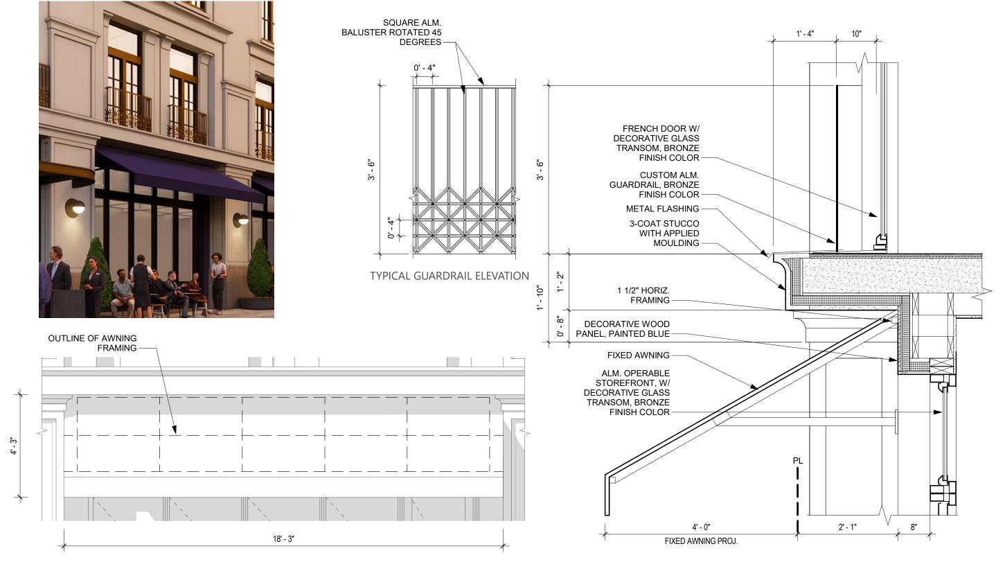
TYPICAL AWNING ELEVATION FIXED AWNING SECTION
