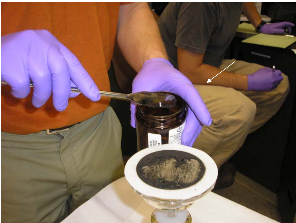
Photo 3 (June 2007). Laboratory setup showing transfer of filtered solids to the sample jar for analytical testing.
