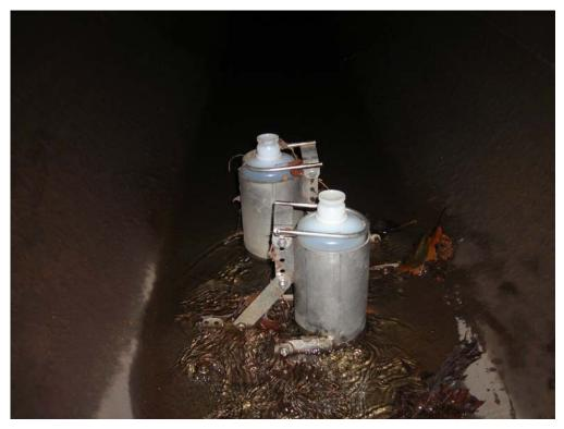
**Photo 14 (October 15, 2007)**: Deployed sediment traps at sampling location ST5; upstream of Manhole AAA170.
