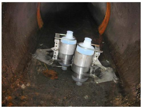
Photo 2 (October 15, 2007): Deployed sediment traps at sampling location ST1
