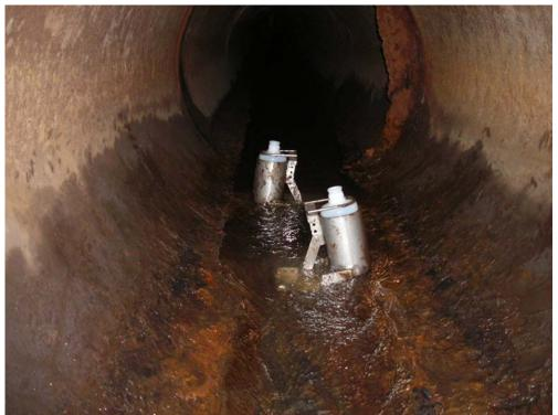
**Photo 6 (October 15, 2007):** Deployed sediment traps at sampling location ST2; upstream of Manhole AAA179 in northern branch.
