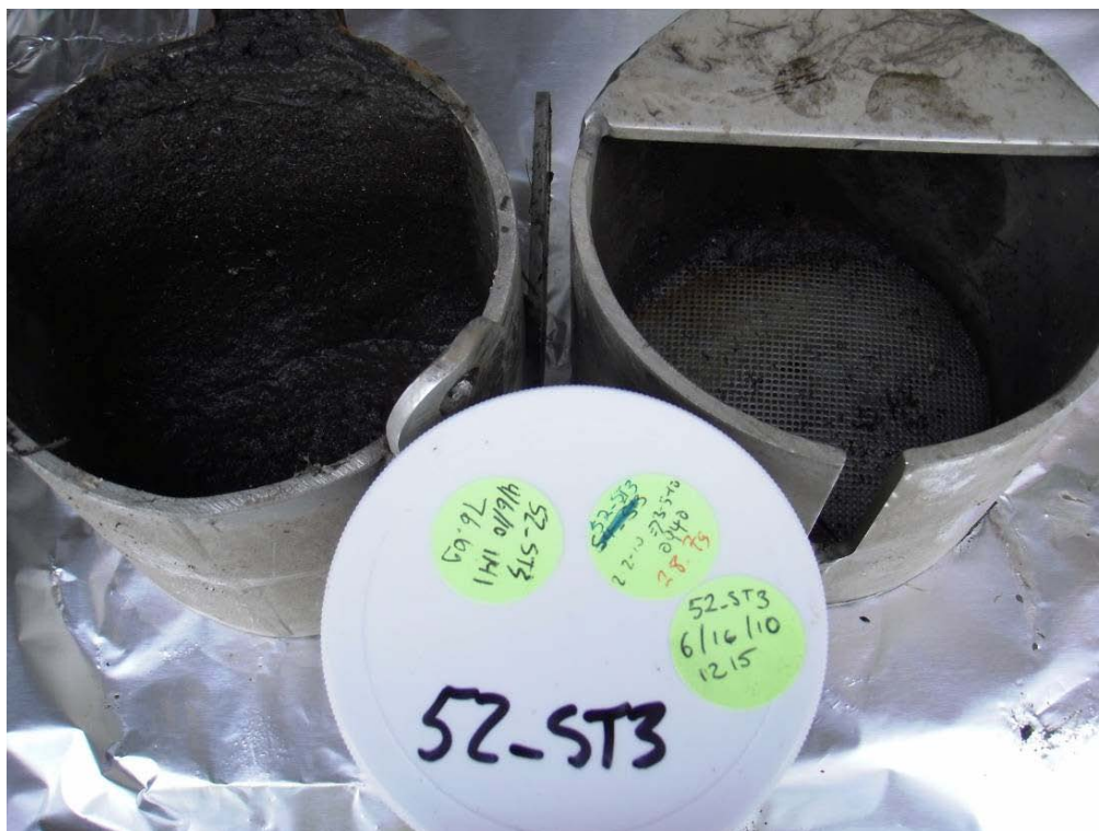
Photo 45 (June 16, 2010). Primary and secondary chambers of SIFT© sediment trap at time of removal.
