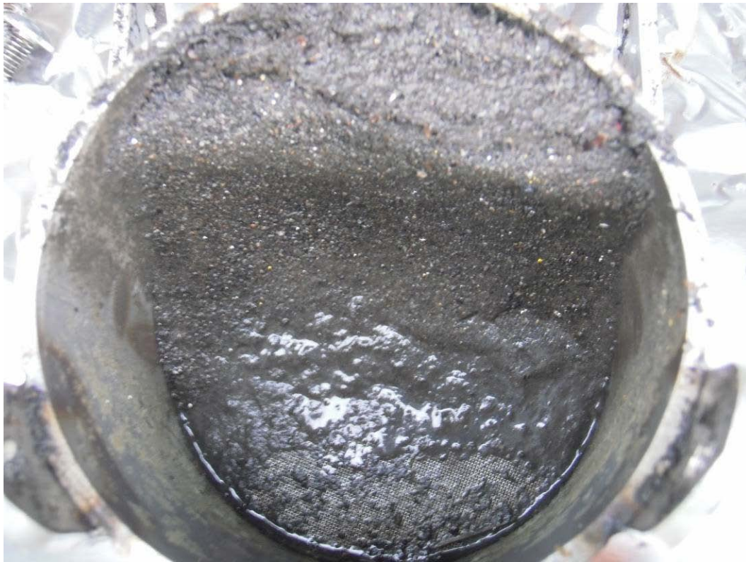
Photo 51 (June 16, 2010). Accumulated sediment in secondary chamber at time of removal.
