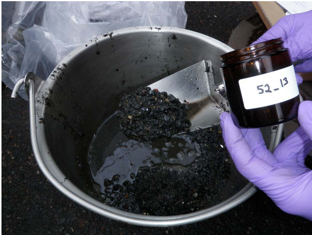
Photo 59 (September 7, 2010). Final homogenized sample from ODOT manhole 2.
