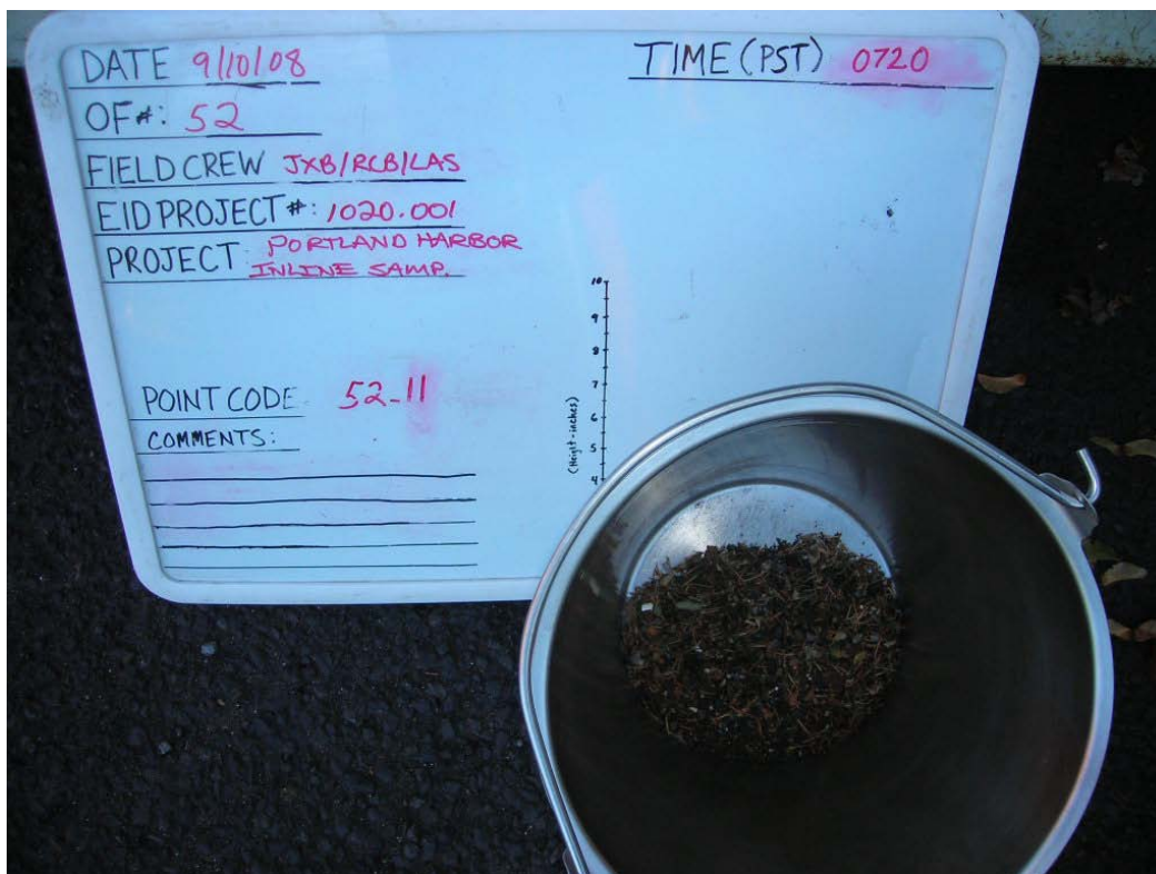
Photo 28 (September 10, 2008). Final composited sample from catch basin ANE910.
