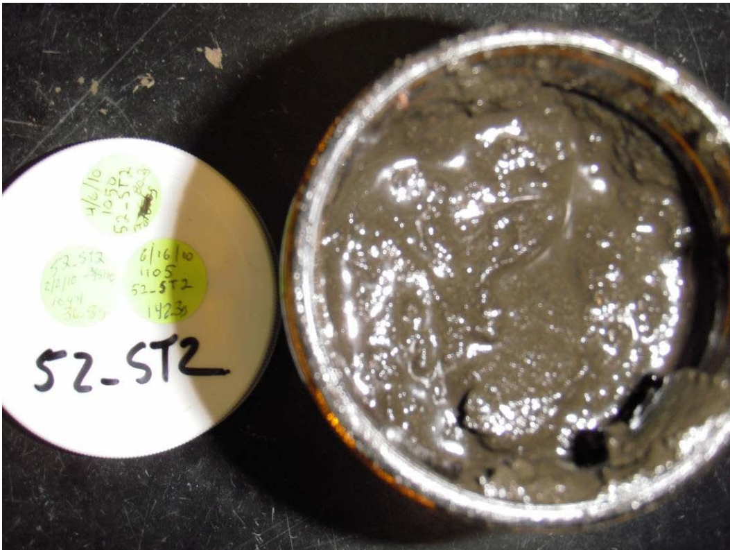
Photo 40 (June 17, 2010). Final homogenized composite sediment trap sample from ST2 / manhole AAE513.
