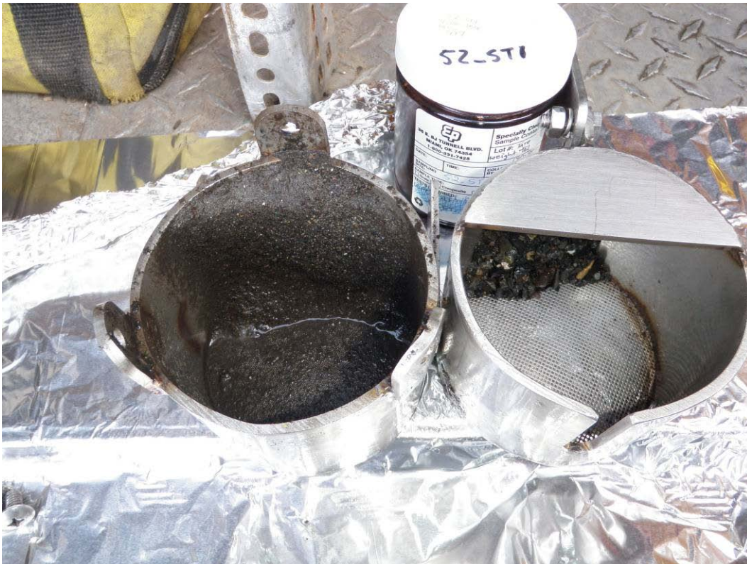
Photo 33 (April 6, 2010). Primary and secondary sediment trap chambers at monthly field check.
