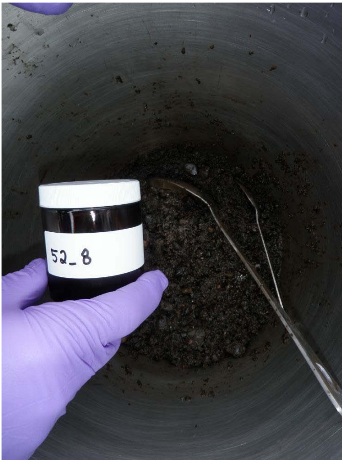
Photo 56 (September 7, 2010). Final homogenized sample from catch basin ANE911.
