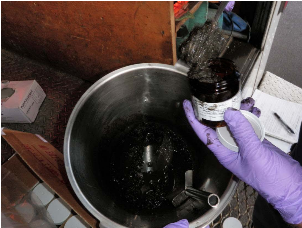
Photo 62 (September 8, 2010). Final homogenized sample from ODOT manhole 4.
