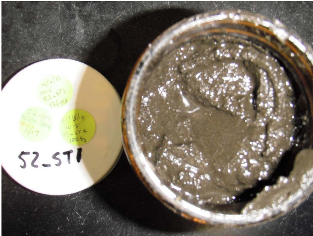
Photo 35 (June 17, 2010). Final homogenized composite sediment trap sample from ST1 / manhole AAE498.
