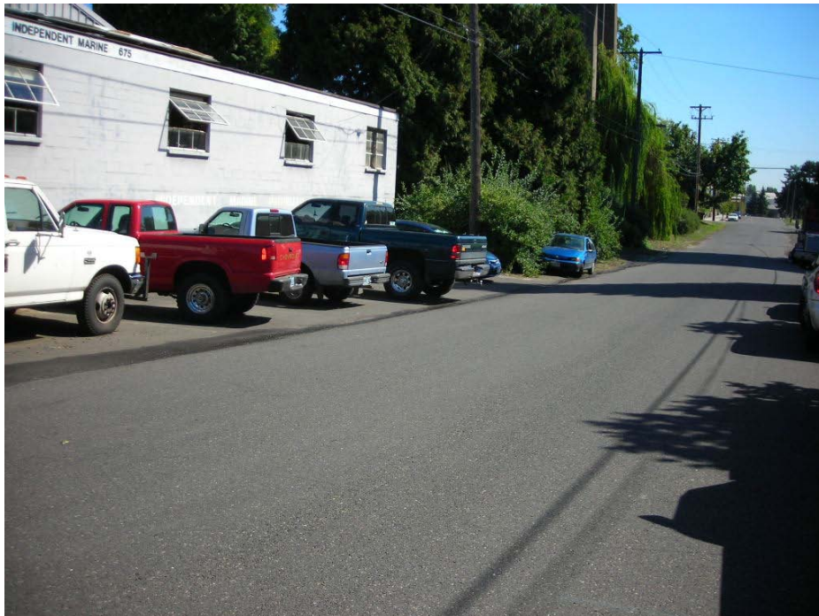
Photo 22 (September 9, 2008). View to the south-southeast on N. Crawford Street, just south-southeast of intersection with N. Alta Avenue. Wash water runoff from Independent Marine Propeller facility driveway is visible along northeast side of roadway, flowing toward catch basin AAE673.
