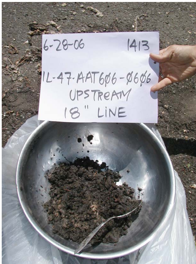
Photo 10 (June 2006). Inline solids collected from the 18-inch-diameter lateral. This sample identification code is AAT606-S.
