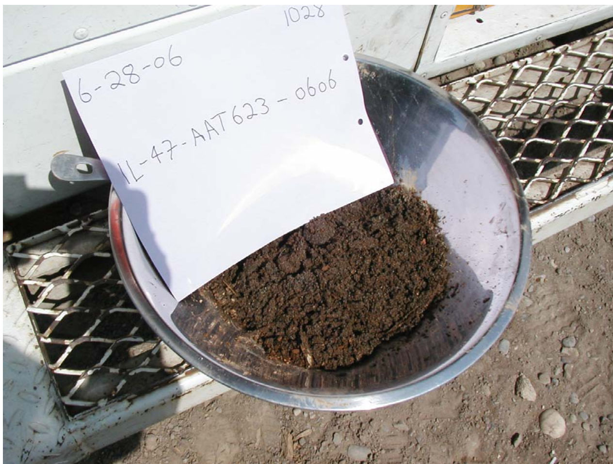
Photo 2 (June 2006). Solids collected from manhole AAT623.
