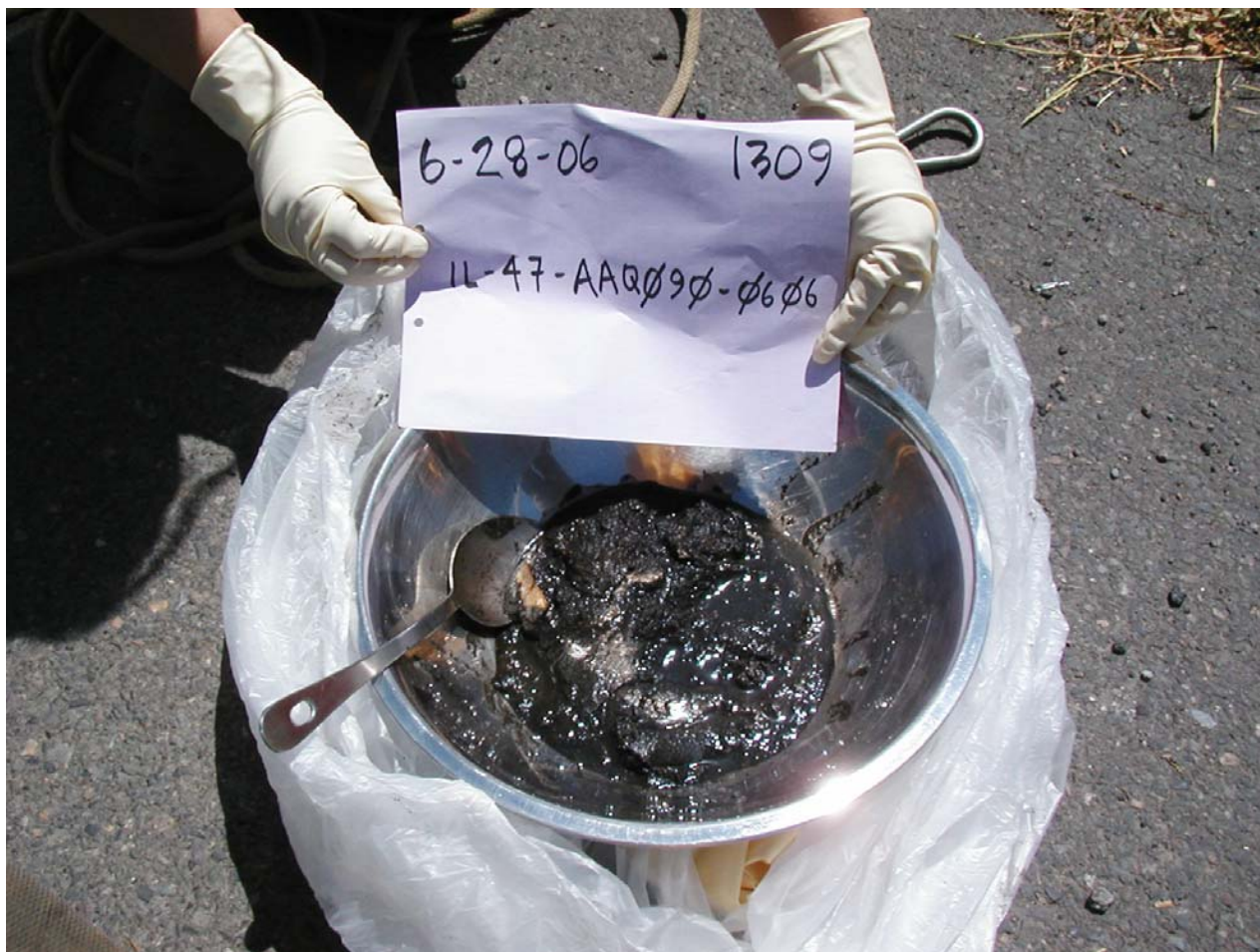
Photo 5 (June 2006). Solids collected from manhole AAQ090.
