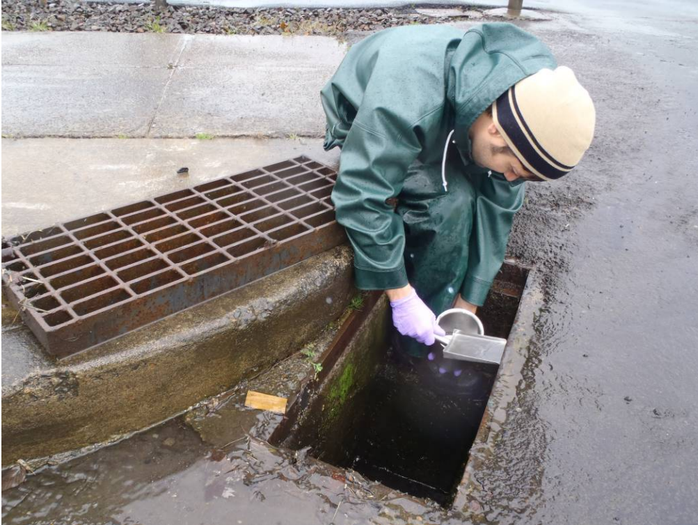
Photo 9 (March 15, 2012). Collecting sample of runoff into catch basin APL246.
