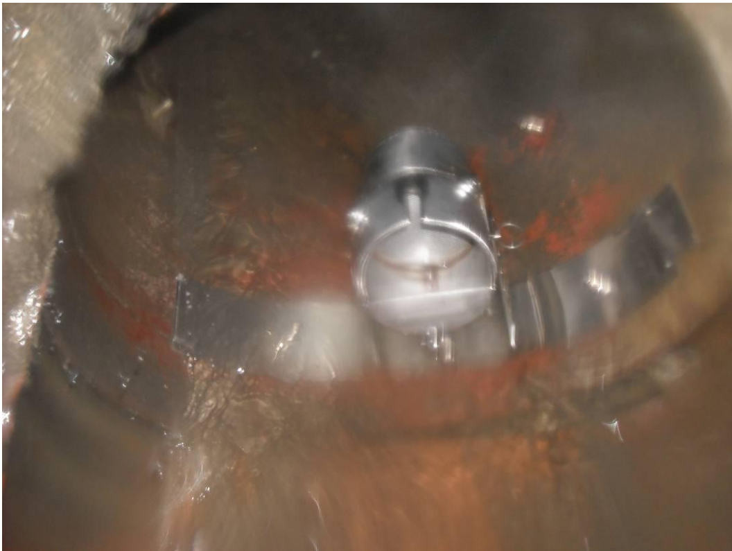
Photo 31 (December 30, 2009). SIFT© type sediment trap deployed at ST6 (downstream of Manhole ABC363 in 16-inch line).
