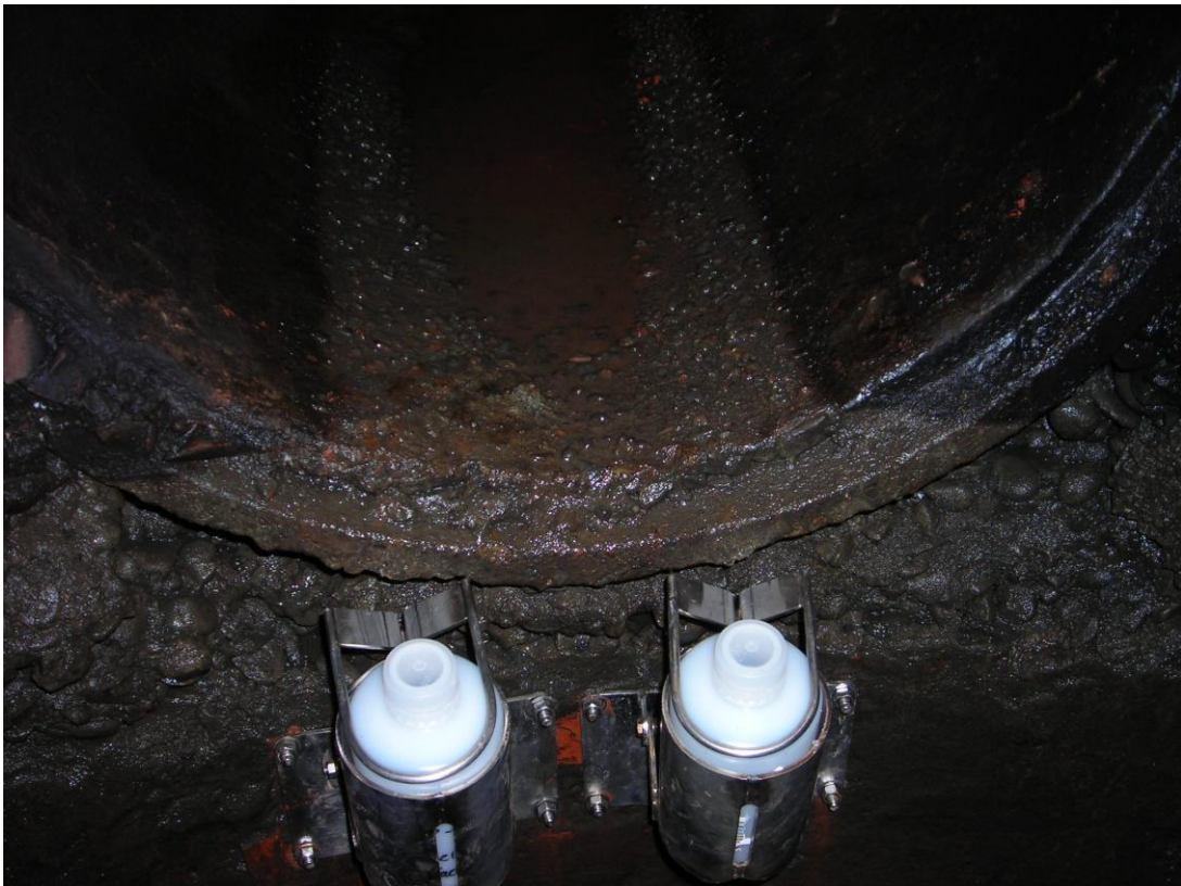
Photo 11 (November 24, 2008). Deployed sediment traps at sampling location ST2 (Manhole ABC539). Traps are mounted on the wall of the manhole, just below the outgoing 27" line.
