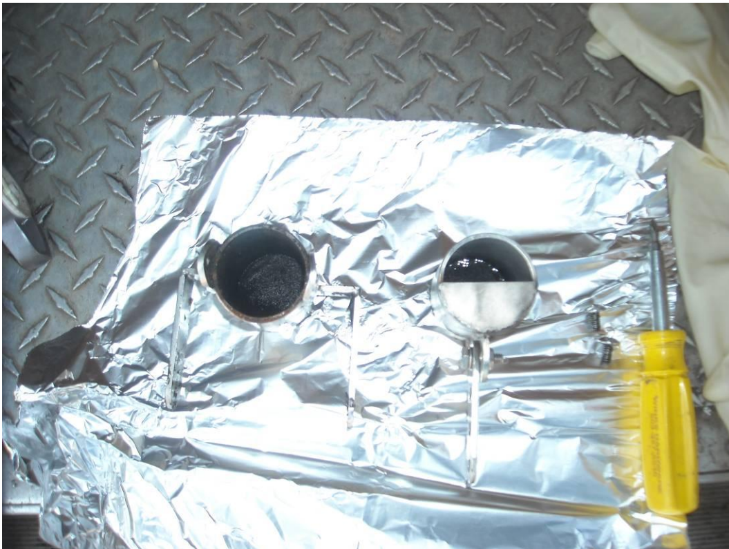
Photo 29 (April 15, 2010). Primary and secondary chambers of SIFT© trap with accumulated solids at time of April 15 field check at ST5 (Manhole ABC270).
