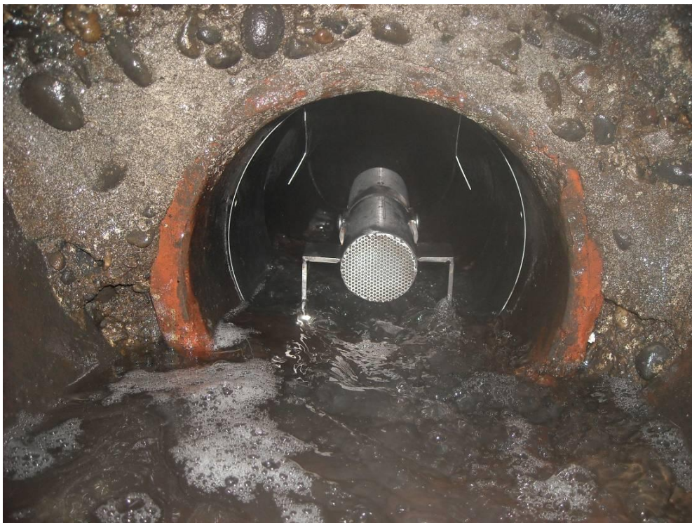
Photo 28 (December 30, 2009). SIFT ©1 sediment trap deployed at ST5 (Manhole ABC270) in incoming 8-inch line.
