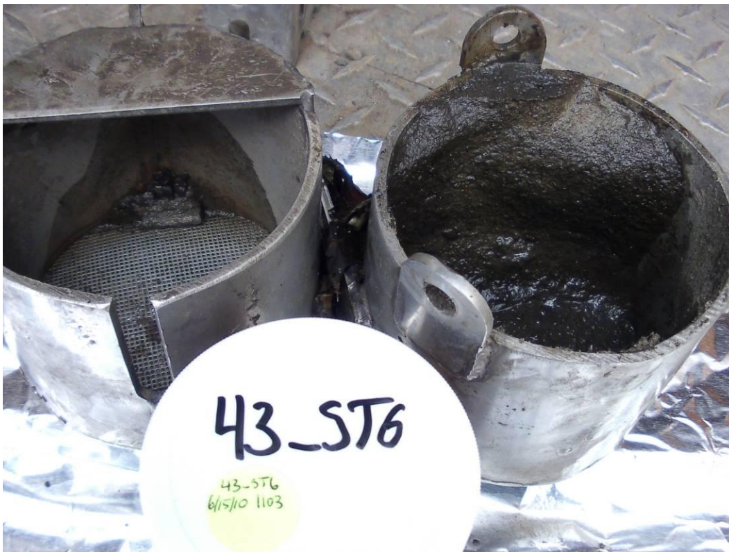
Photo 33 (June 15, 2010). Solids present in secondary chamber in SIFT© sediment trap from ST6 (Manhole ABC363) at time of trap removal.
