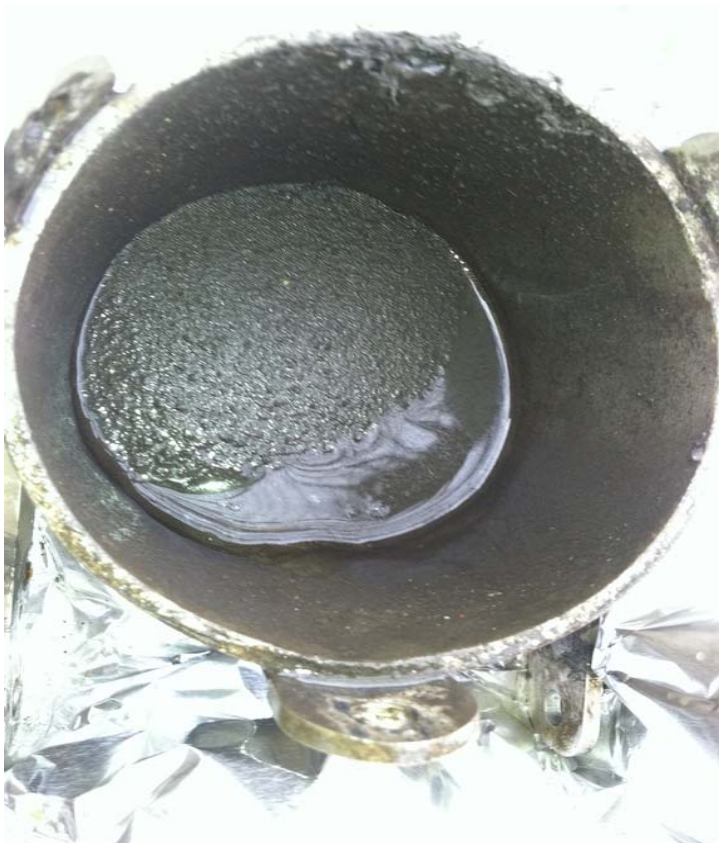
Photo 8 (May 23, 2011). Secondary trap chamber and accumulated solids during monthly field check at sample location ST7 (Manhole AAX278).
