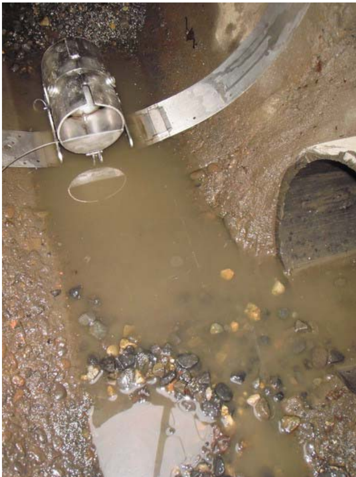
Photo 2 (December 21, 2010). Deployed SIFT© sediment trap at sampling location ST6 (Manhole AAX318).
