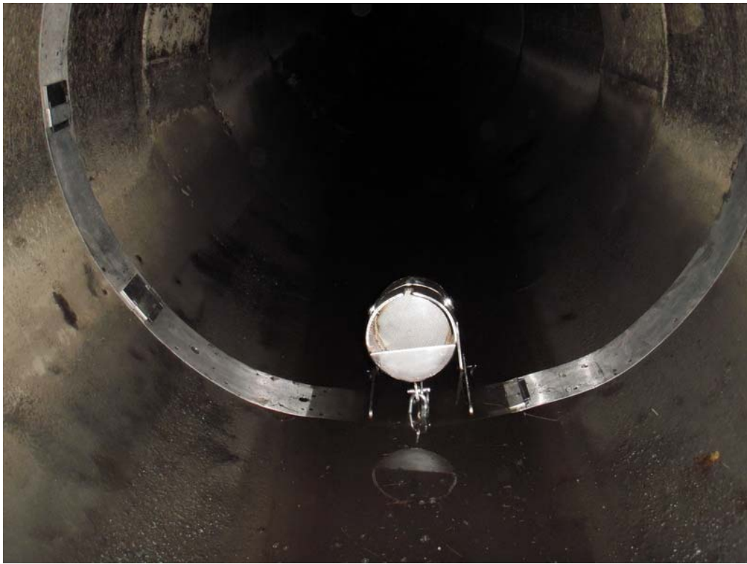
Photo 7 (December 21, 2010). Deployed SIFT© sediment trap in the outgoing 30-inch line at Manhole AAX278 (ST7).
