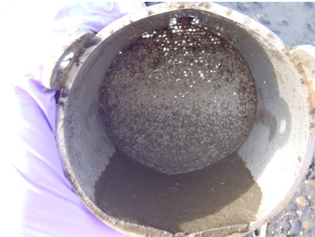
Photo 4 (January 26, 2011). Secondary trap chamber and accumulated solids at time of first monthly field check.
