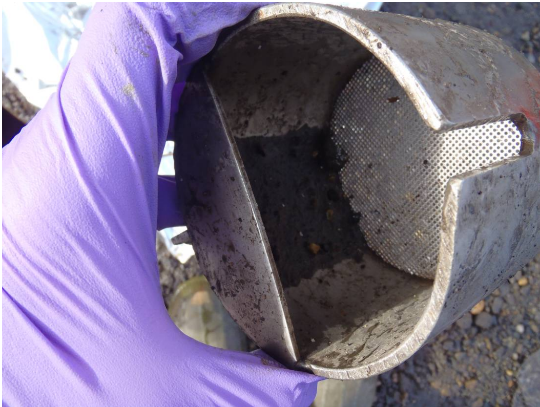
Photo 3 (January 26, 2011). Primary trap chamber and accumulated solids at time of first monthly field check.
