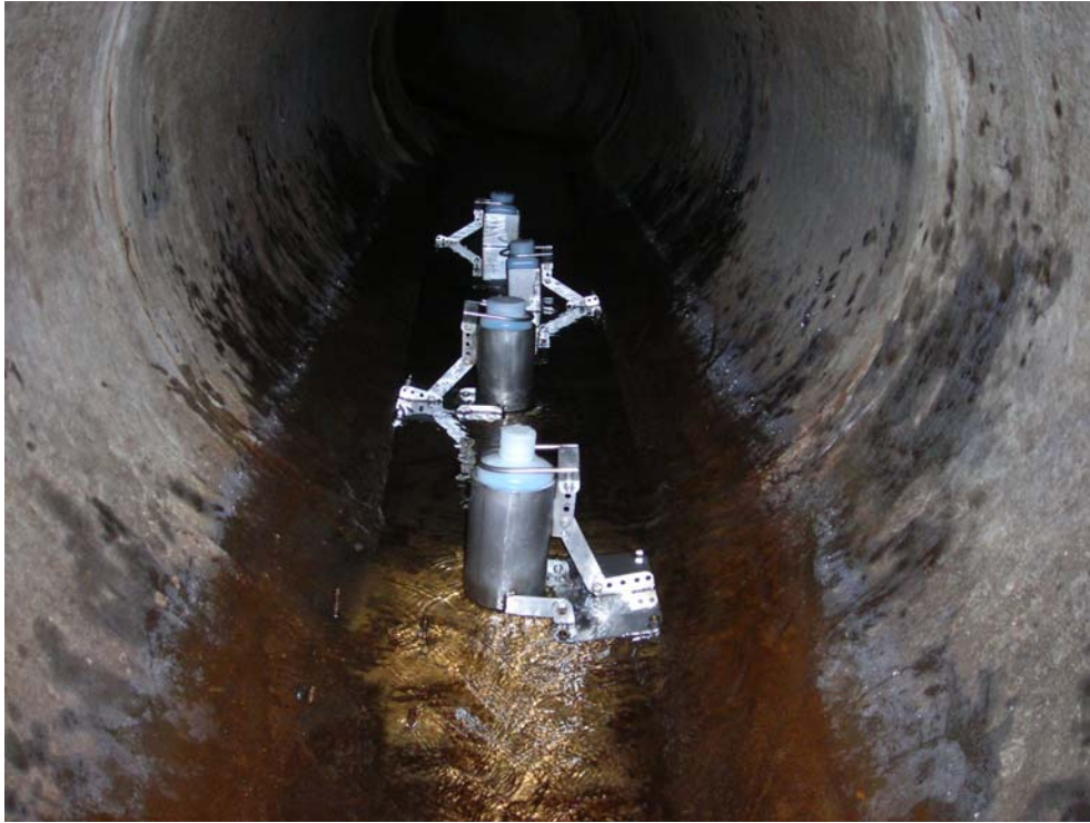
Photo 9 (December 2008). Western Subbasin sampling location ST3 (Manhole AND535) and installed sediment traps. The trap in the foreground is the furthest downstream.
