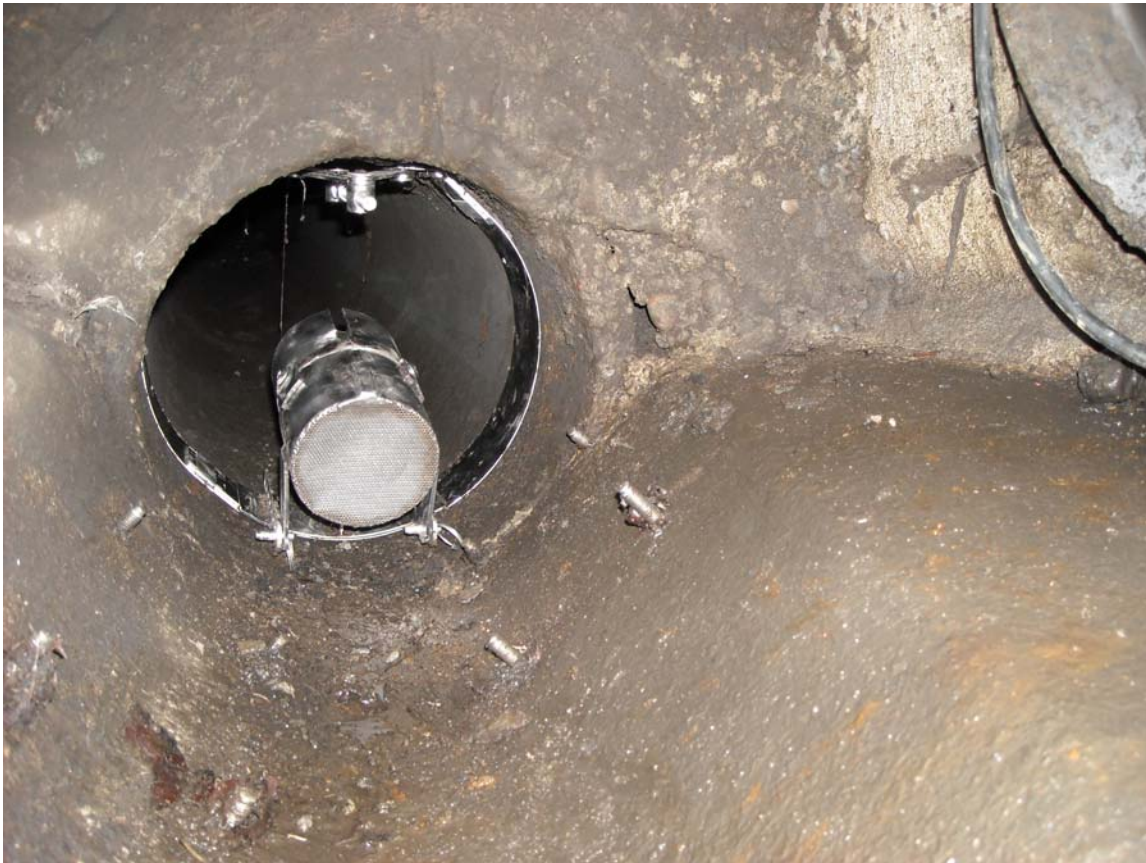
Photo 1: SIFT sediment trap prototype in-situ at location 18_ST1.
