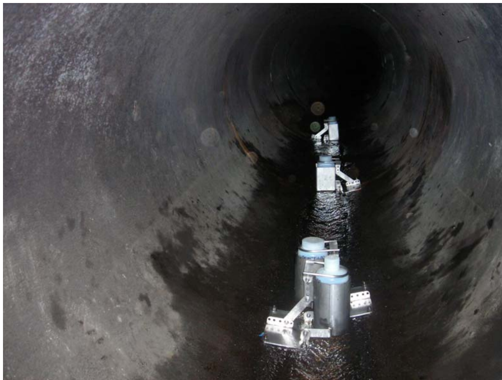
Photo 11 (October 2008). East-Central Subbasin sampling location ST2 (Manhole AAT557) and installed sediment traps. The trap in the foreground is the furthest downstream.
