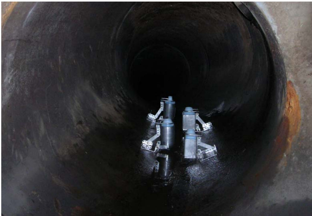
Photo 10 (December 2008). West-Central Subbasin sampling location ST4 (Manhole AAT466) and installed sediment traps. The trap in the foreground is the furthest upstream.
