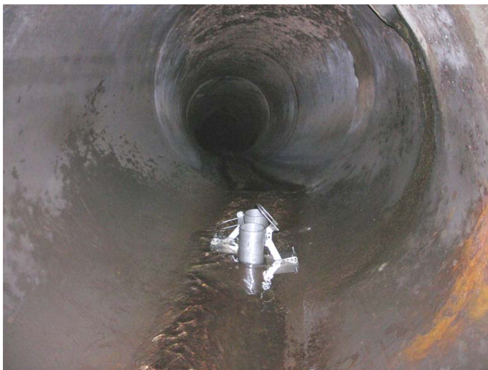
Photo 4 (June 2007). Installed sediment traps at sampling location ST4.
