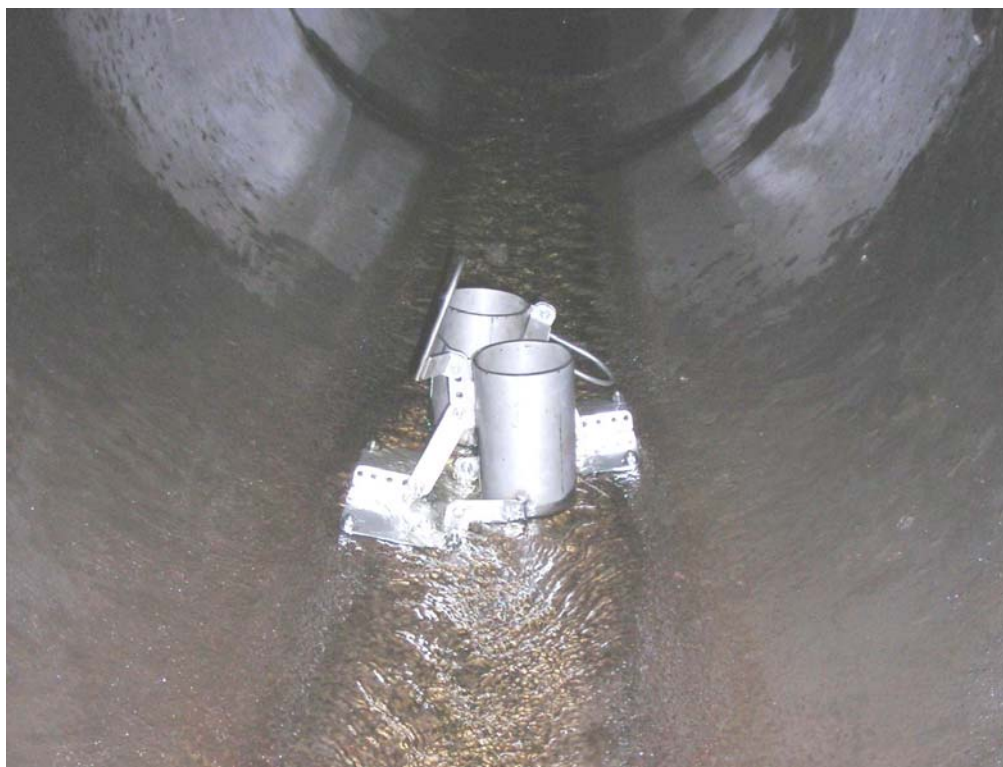
Photo 6 (June 2007). Installed sediment traps at sampling location ST2.
