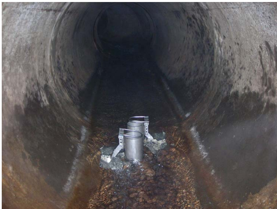
Photo 2 (June 2007). Installed sediment traps at sampling location ST3.
