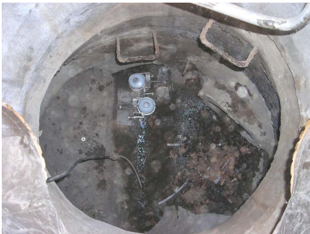
Photo 8 (June 2007). Installed sediment traps at sampling location ST1.
