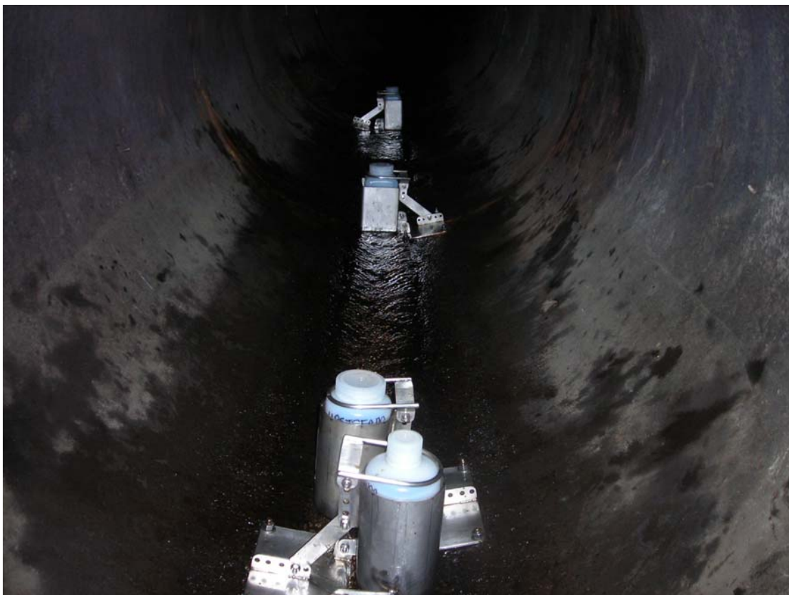
Photo 2: Trap orientation at location 18_ST2; the trap at the top of the photo is the furthest upstream.
