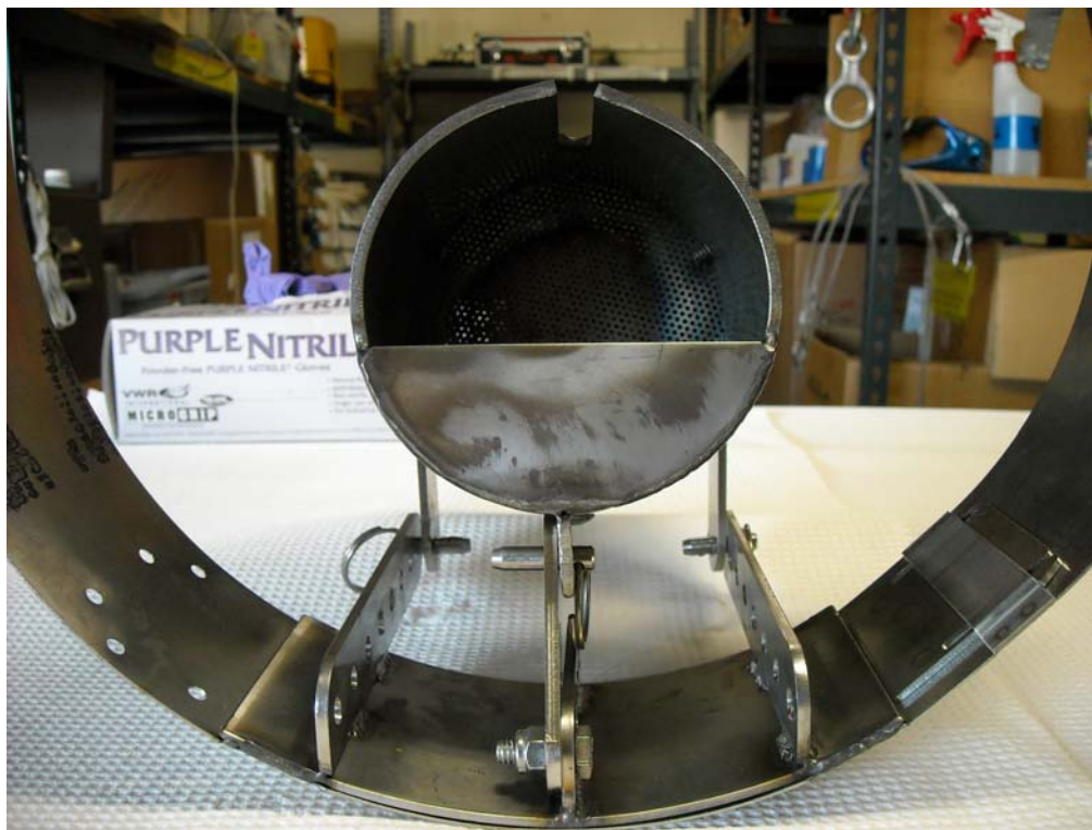
Photo 14. Flow-through sediment trap during development, subsequently installed in eastern subbasin sampling location ST1 (Manhole AAT565).
