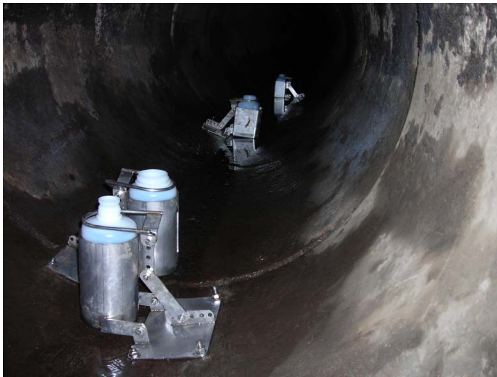
Photo 13 (December 2008). East-Central Subbasin sampling location ST5 (Manhole AAX261) and installed sediment traps. The trap in the foreground is the furthest downstream.
