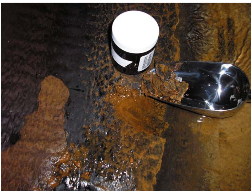
Photo 11 (November, 2005). Solids had to be scraped from the main line through manhole AMZ116. Note the color of the sample indicating iron-oxide precipitate.
