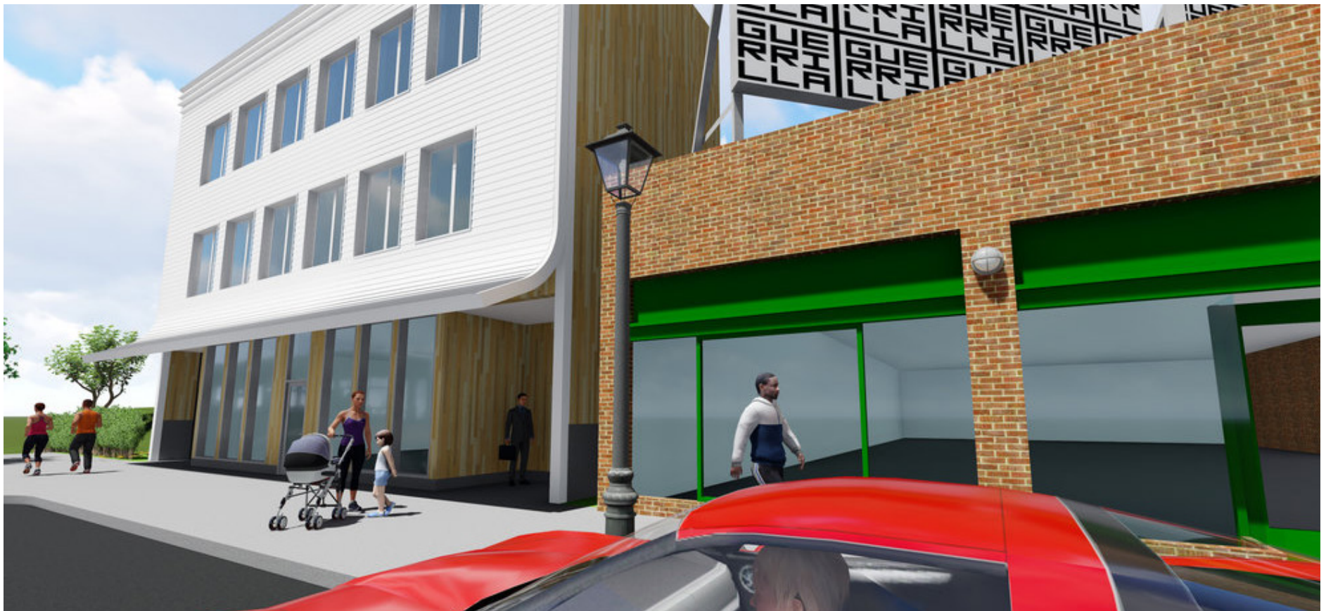
Rendering of a new mixed-use building (at left) in North Portland. The new building employs a tall ground floor height to match the ground floor height of the existing building (at right). Image courtesy Guerrilla Development.
