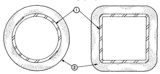
1. Steel Pipe or Tube Column — Steel circular pipe (SP) with diameter (ID) ranging from a minimum of 3 in. to a maximum of 32 in. with a minimum wall thickness of 3/16 in.
