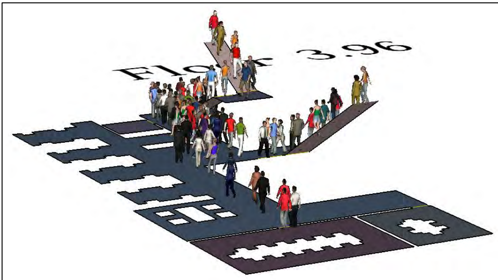
Figure 10: Second Floor Plan – 46.9 seconds into egress, the occupants use both the enclosed interior exit stair and the unenclosed exit access stair for egress.
