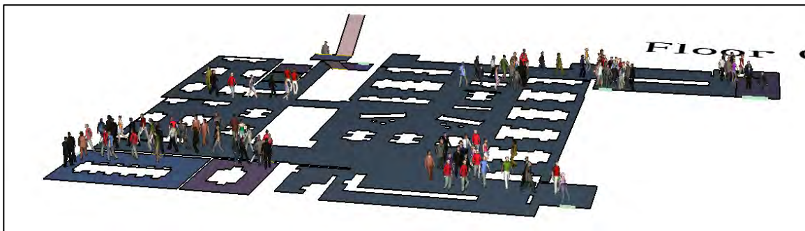
Figure 6: First Floor Plan – 12.2 seconds into egress, the occupants disperse to various exits.
