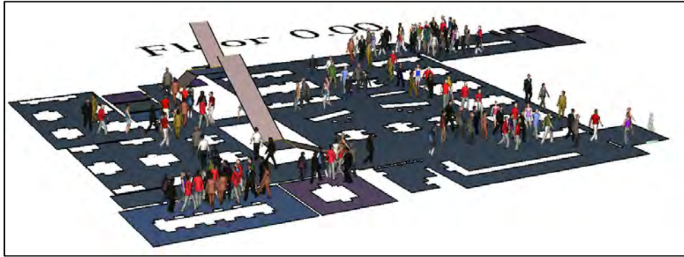
Figure 9: First Floor Plan – 9.6 seconds into egress, the occupants use either of the two exits.
