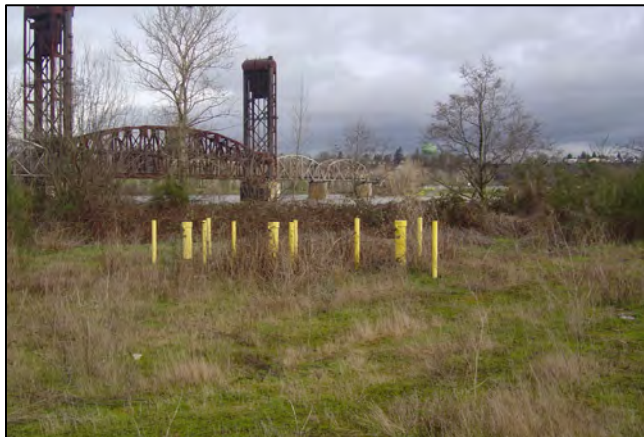
Groundwater monitoring wells measure contaminant levels at a former pesticide manufacturing facility.
