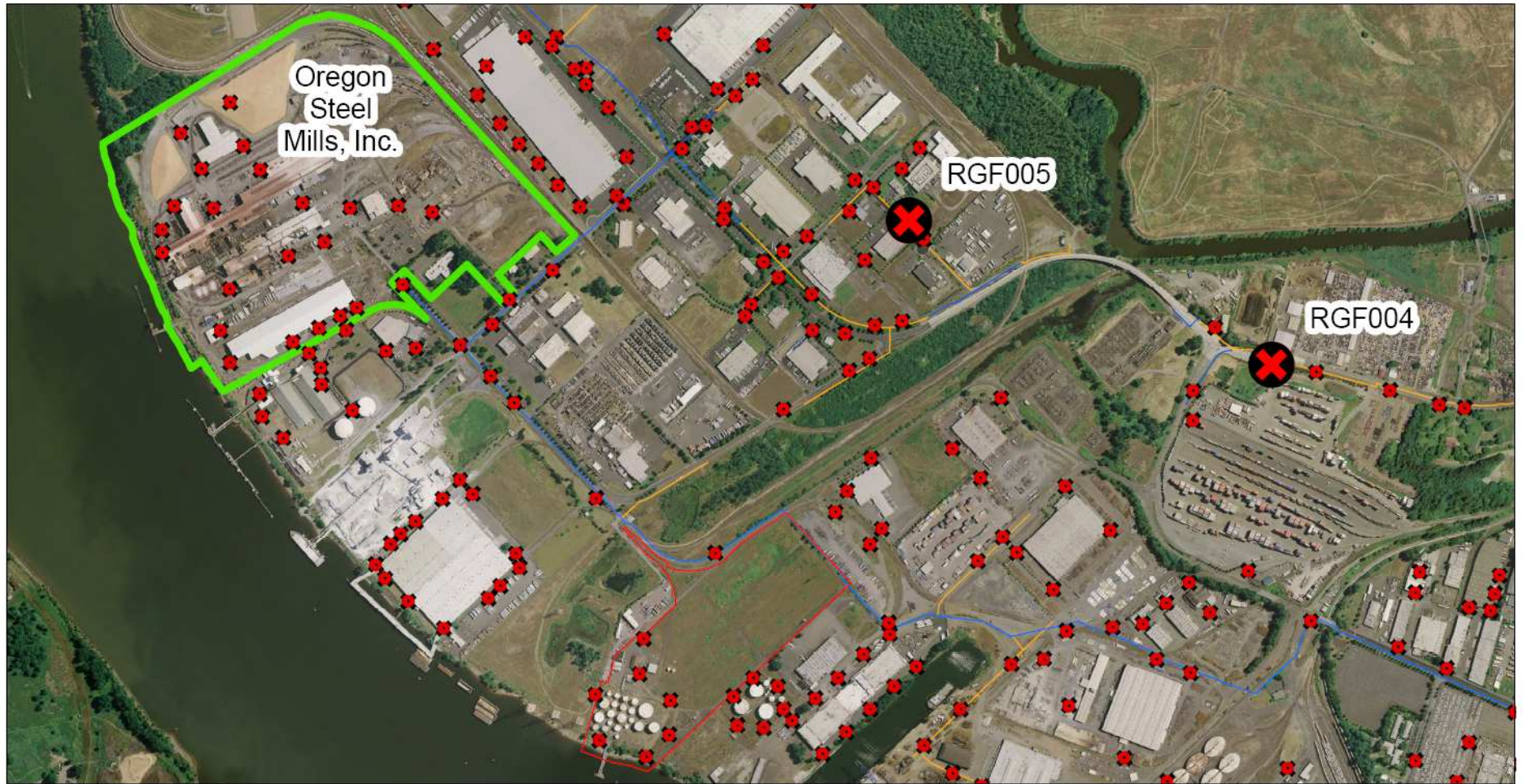
Figure 40. Hydrant Spacing Clustered Around Structures at Oregon Steel Mills, Inc.
