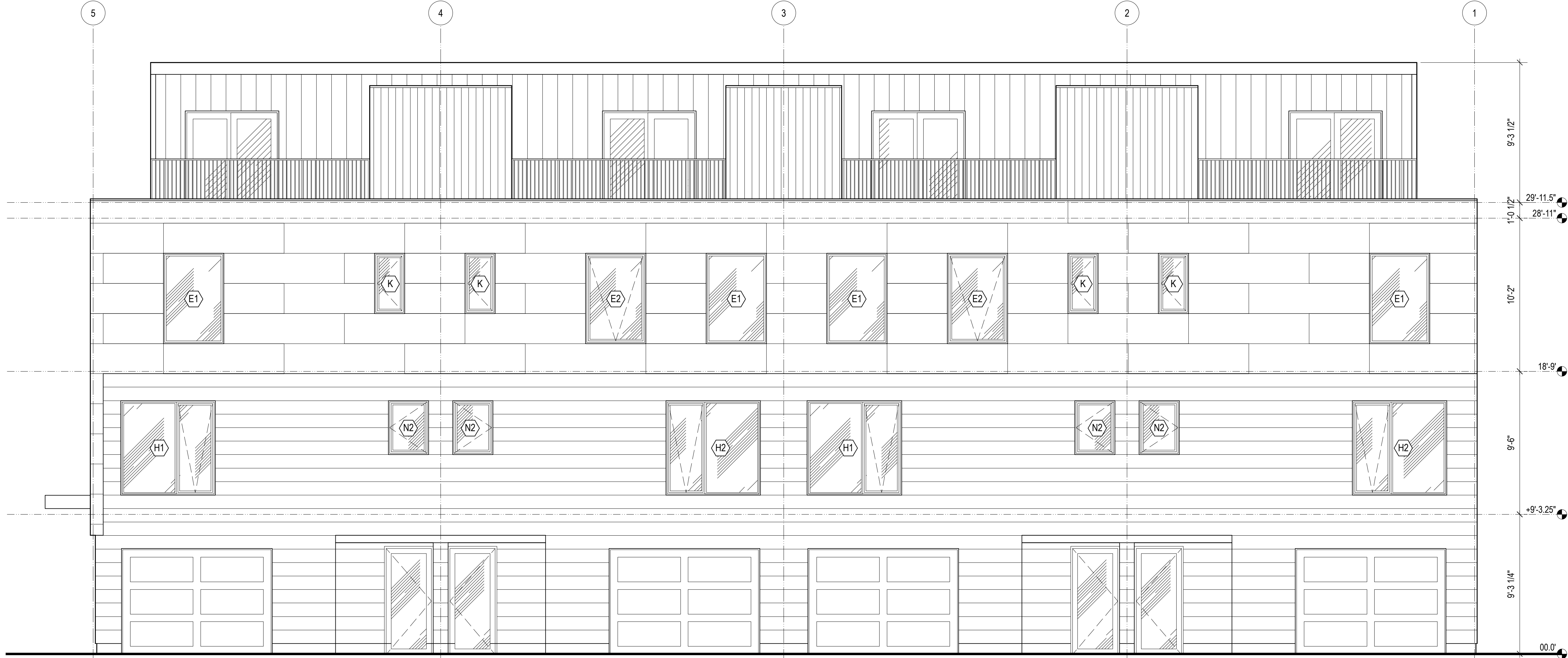
2 EAST BUILDING - West Elevation Scale: 1/4" = 1'-0"
