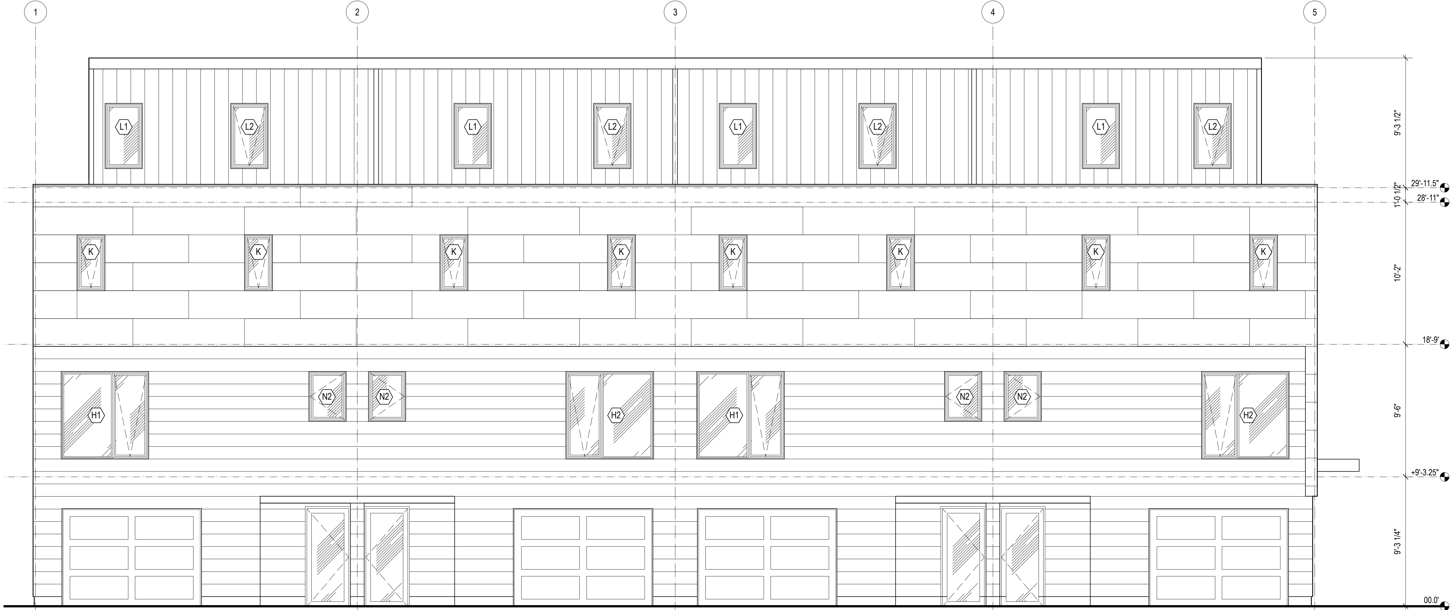
2 WEST BUILDING - East Elevation Scale: 1/4" = 1'-0"
