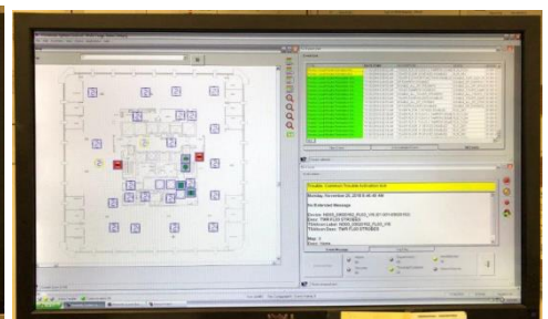
Figure 7 - Floor View Indicating Location and Type of Initiating Device
