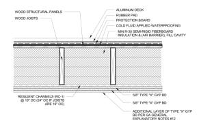
R7 1 HR RATED ROOF-CEILING ASSEMBLY BASED ON GA FILE 5529
