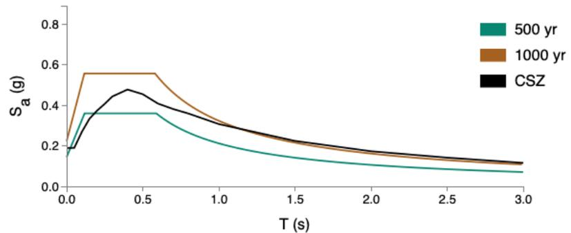
Figure 10: Spectral Acceleration for Portland's CEI Hub
