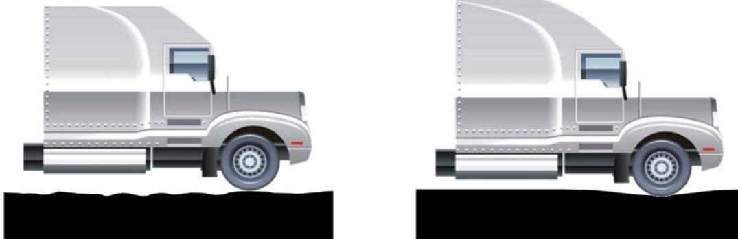
MIT has developed models that quantify excess fuel consumption due to pavement-vehicle interaction for pavement segments and pavement networks
