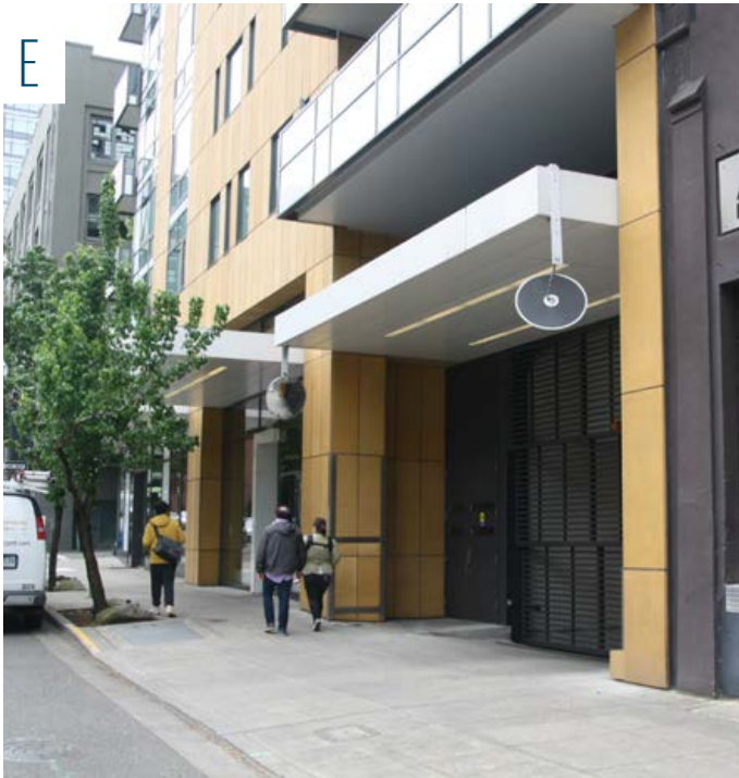
Following the rhythm of storefront and entry bays in the placement of openings for structured or underground parking. Pearl, NW 12th and NW Everett
