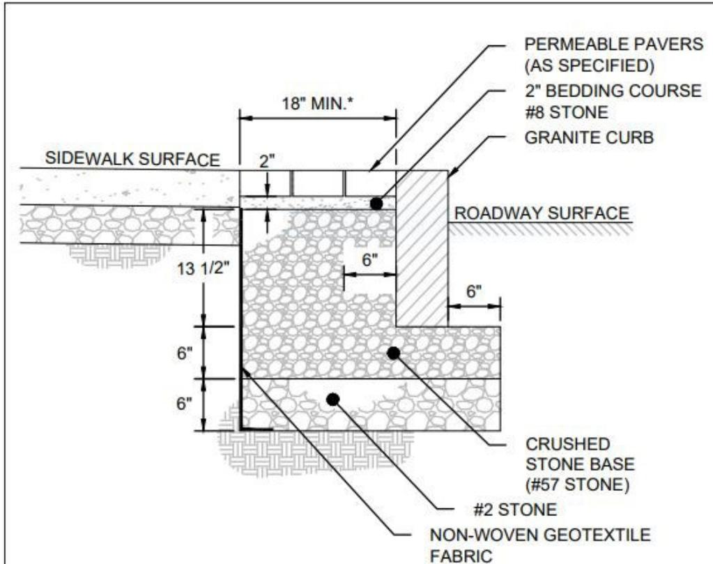
\*PERMEABLE PAVERS SHALL BE INSTALLED WITH A MINIMUM WIDTH OF 18" FOR SIDEWALKS UP TO 7'. FOR SIDEWALKS OVER 7', PERMEABLE PAVER WIDTH SHALL BE 1' PER 5' OF SIDEWALK.
