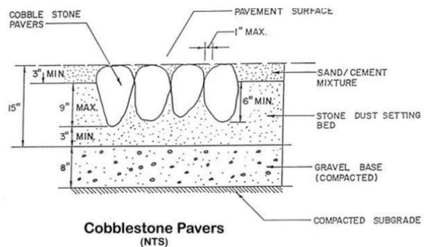
Figure 4. Detail of suggested Cobblestone Pavers in Nantucket, MA.
