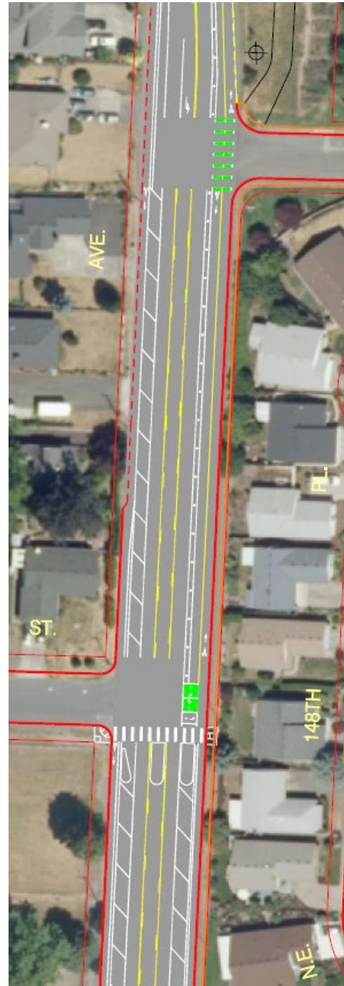
Figure 12 - Striping concept for NE 148th Avenue at the offset crossing of NE Sacramento Street.
