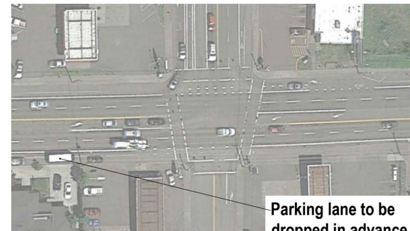
Parking lane to be dropped in advance of driveway and intersection; widen bike lane and buffer. Exact treatment to be determined in future design phases.
