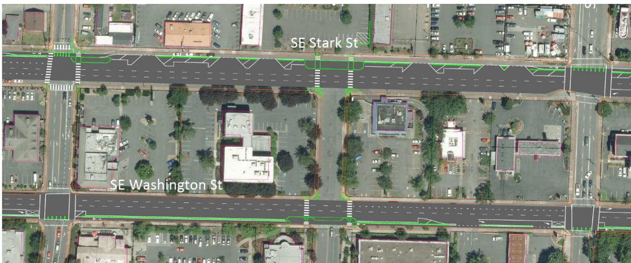
Figure 6 - Project concept on SE Stark and Washington Streets, shown here between SE 99th and 102nd Avenues. Improvements include pedestrian crossings, protected bike lanes and transit islands.
