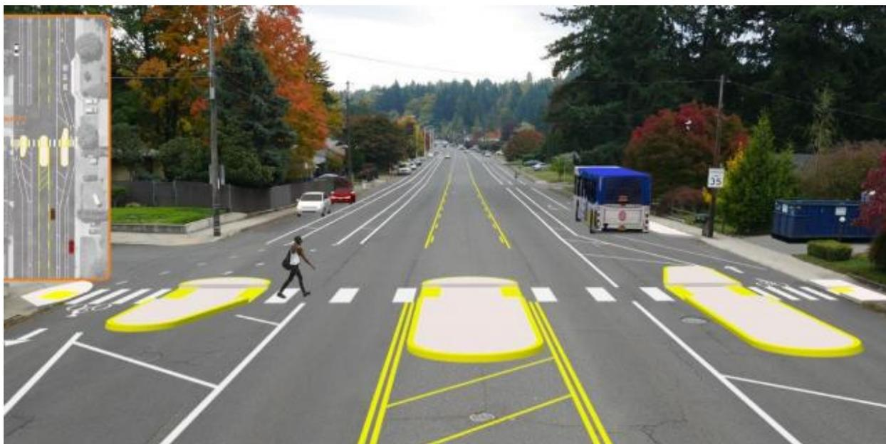
Figure 13 - Illustration of proposed pedestrian crossing at SE 162nd Avenue at SE Tibbetts Street, including 5-to-3-lane road reorg.
