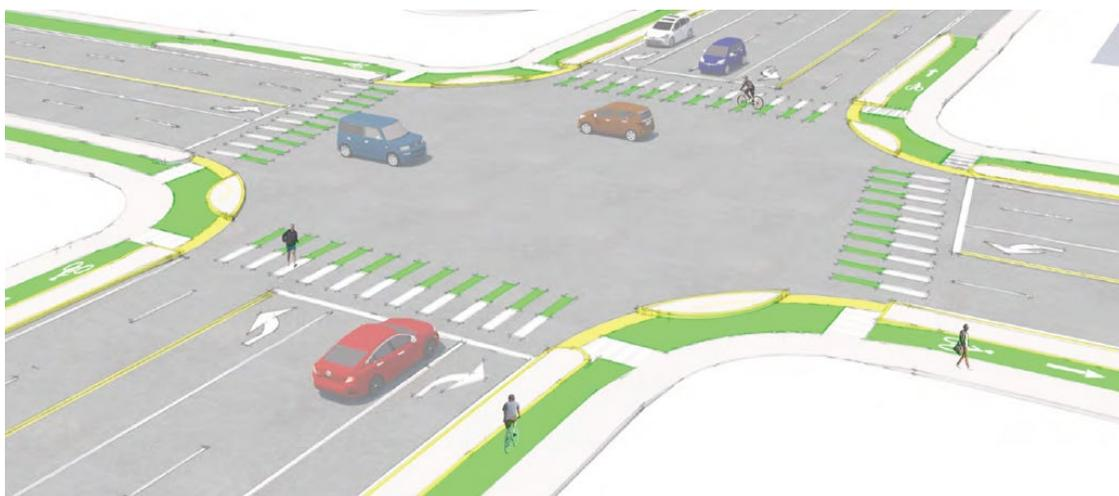
Figure 7 - A “protected intersection” design at SE Stark and 122nd Avenue would transform Portland’s most crash-prone intersection.
