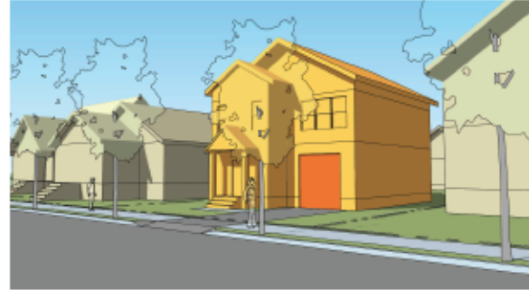
Wider building facades (22 feet or wider) would be allowed to have a garage.
