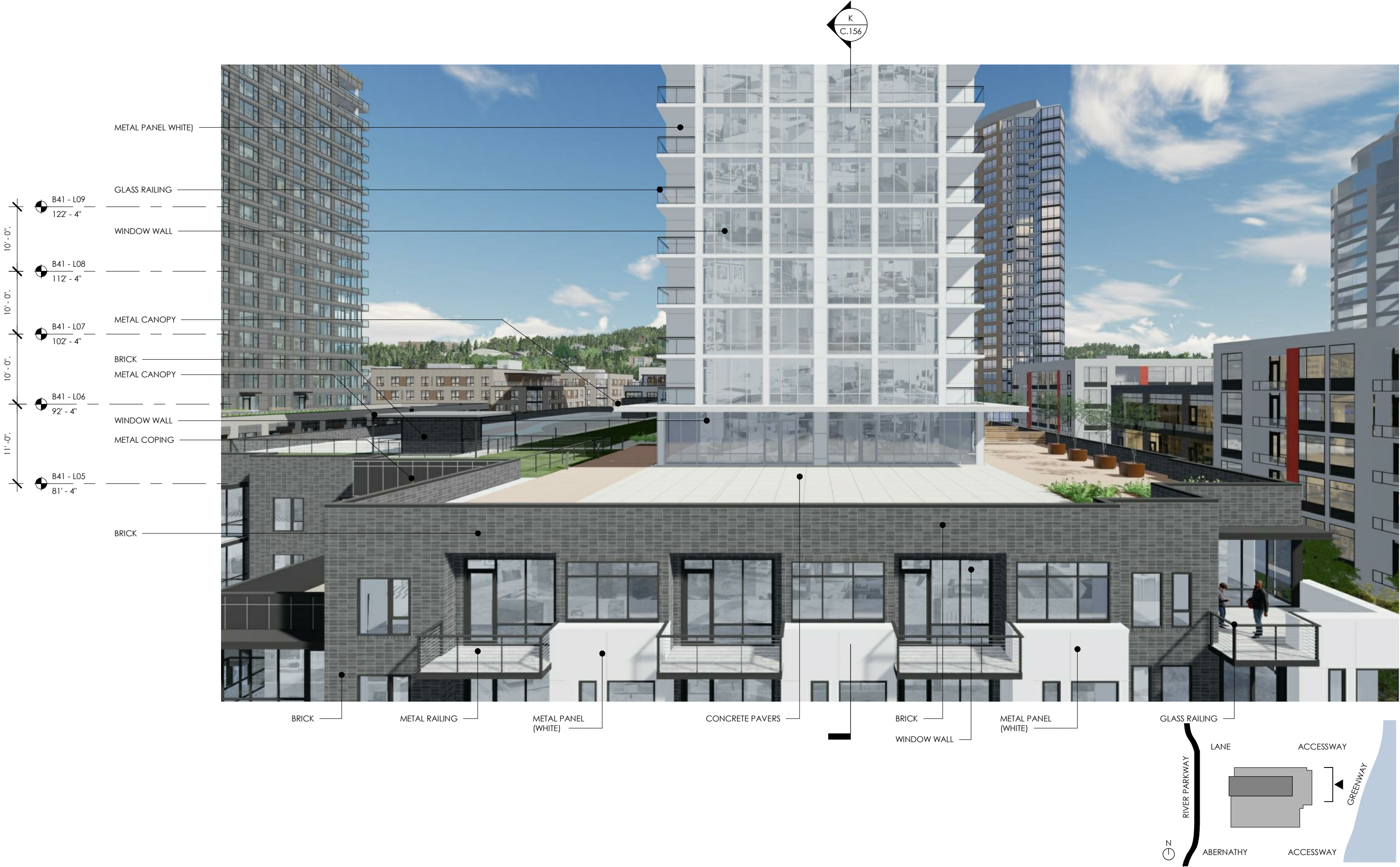
BLOCK 41 - ENLARGED ELEVATION LEVEL 5 AMENITY
