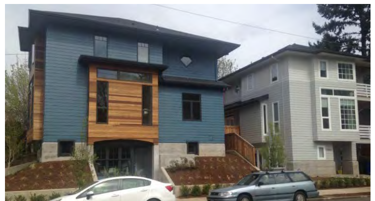
Wider eaves reduce the perceived scale of a house. Bay window projections can also help break up the massing of building walls.
