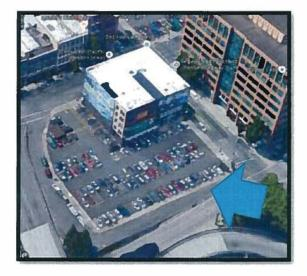
As shown below, the auto circulation lane on SW 1<sup>st</sup> Avenue at this location is physically segregated from the light rail alignment due to the grade change as the light rail alignment dips below the Morrison Bridge ramps adjacent to SW Washington.
